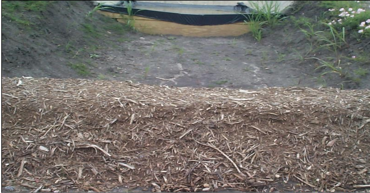
Figure 4.10. Yard Waste Compost Berm before Starting the Structural Testing.
