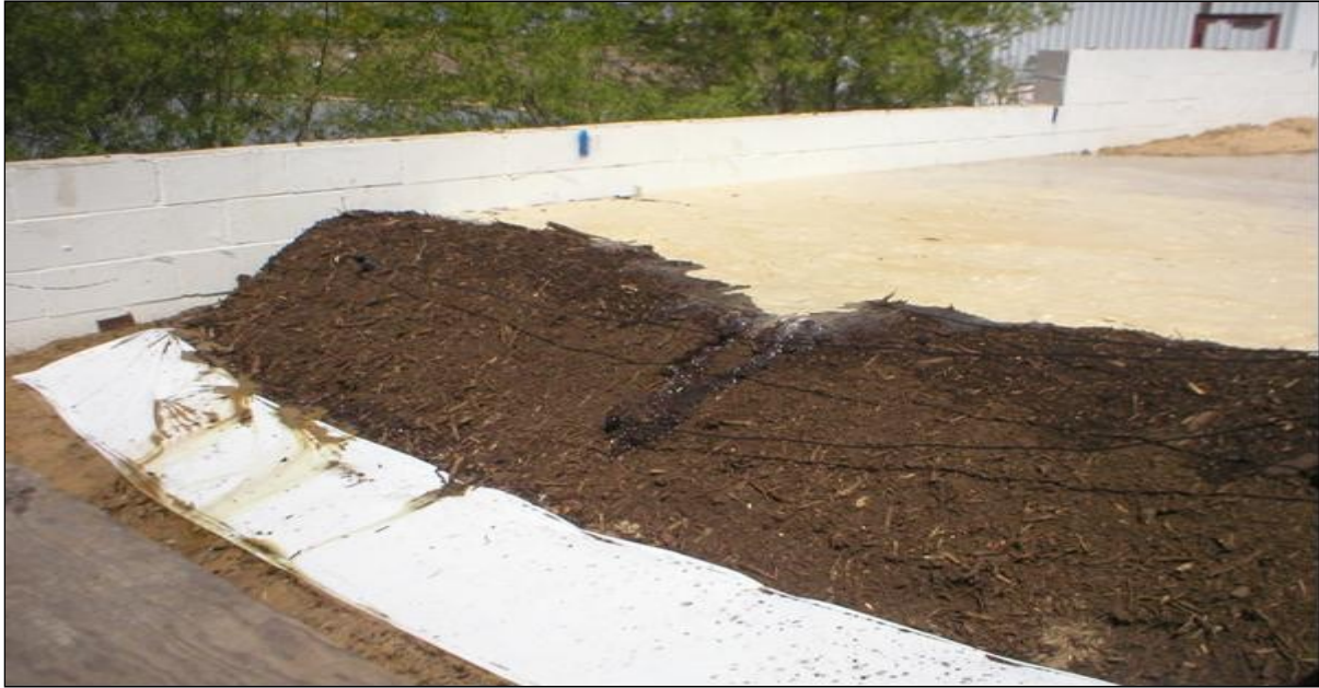
Figure 4.6. Compaction of the Berm Leading to Overtopping with Very Little Infiltration.
