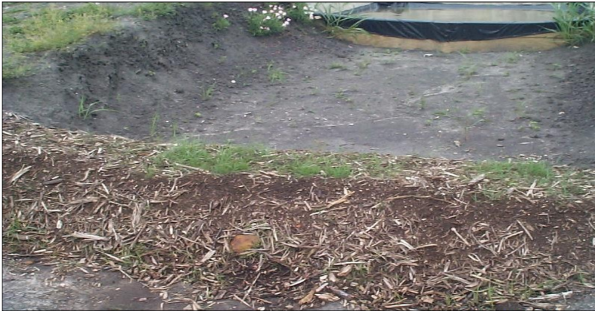
Figure 4.9. Dairy Manure Compost Berm before Starting the Structural Testing.
