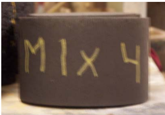
Figure 26. Gyratory Compacted Specimen.
