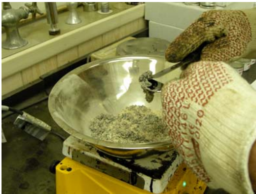
Figure 22. Mixing Binder-Filler Mixture with Aggregates.
