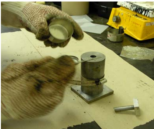
Figure 24. Placing Mixture in Mold.
