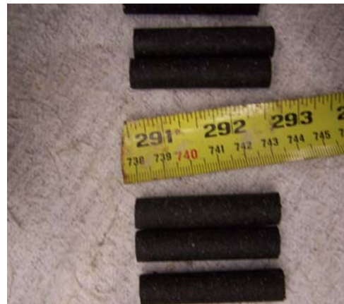
Figure 25. Completed DMA Specimen.
