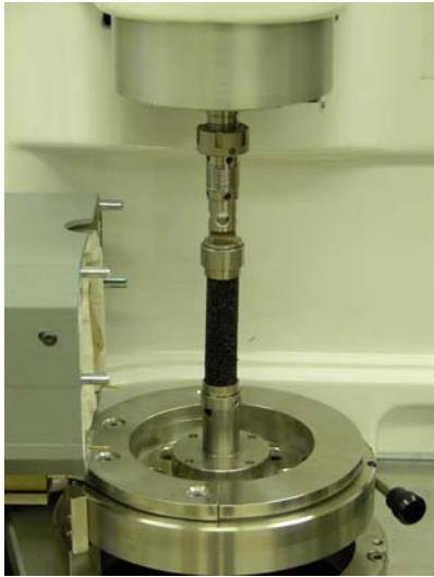
Figure 29. Sample Mounted in DMA.
