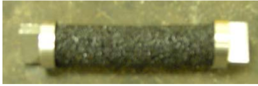
Figure 28. Specimen Placed in Sample Holders for DMA Testing.
