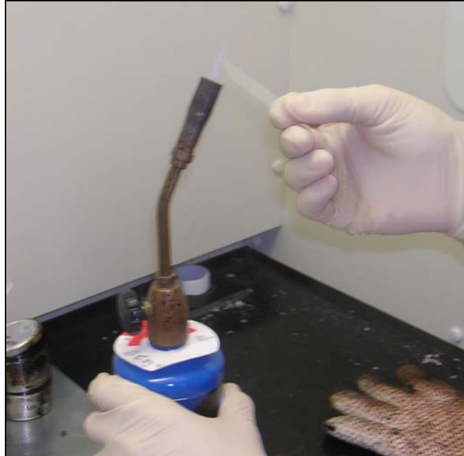
Figure D.2. Glass Slide Dried before Immersion by Passing it over a Propane Flame.
