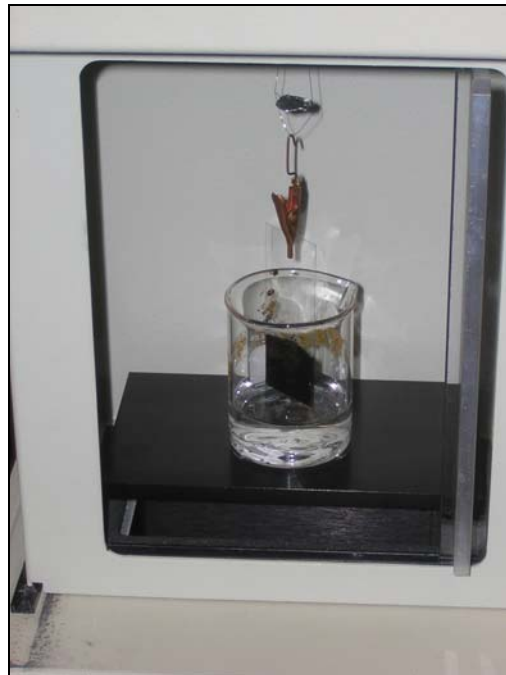
Figure D.6. Asphalt Binder Sample Suspended from Microbalance for Immersion in Probe Liquid.
