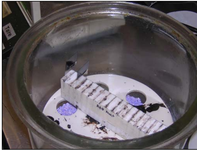
Figure D.5. Finished Slides Stored on Slotted Holder in Desiccator Prior to Testing.
