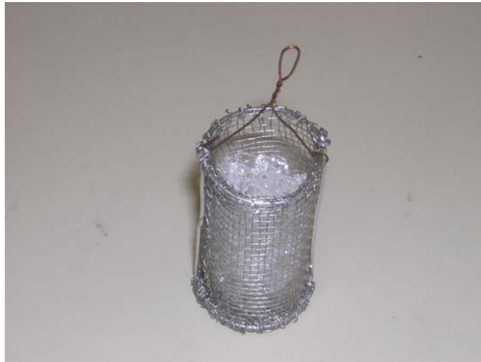
Figure E.2. Basket with Aggregate Sample for Testing with the USD.
