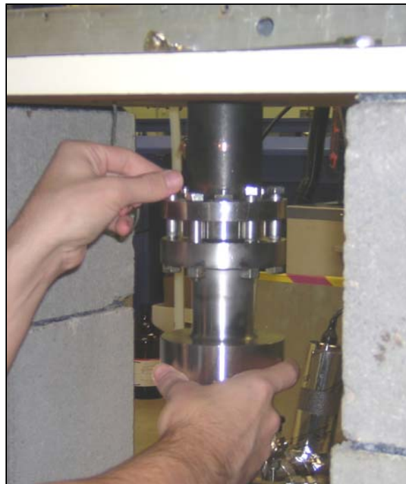
Figure E.4. Adsorption Cell Raised and Sealed with Sample Basket Inside.
