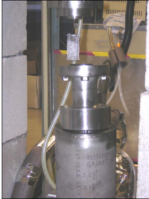
Figure E.3. Sample Basket Suspended from the Magnetic Suspension Balance.
