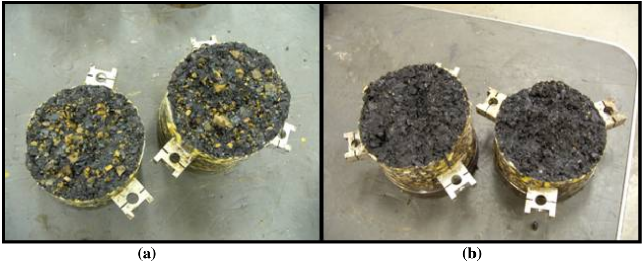
Figure 6.2. Failed Specimens after Tensile Strength Test (a) Wet Specimens Showing Stripping and (b) Dry Specimens Showing Well-Coated Aggregates.
