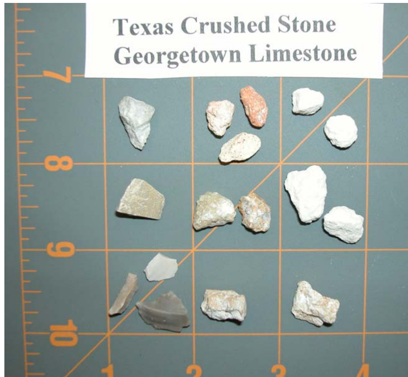
Figure 18. Partitioning of Aggregates Based on Textural Variations.
