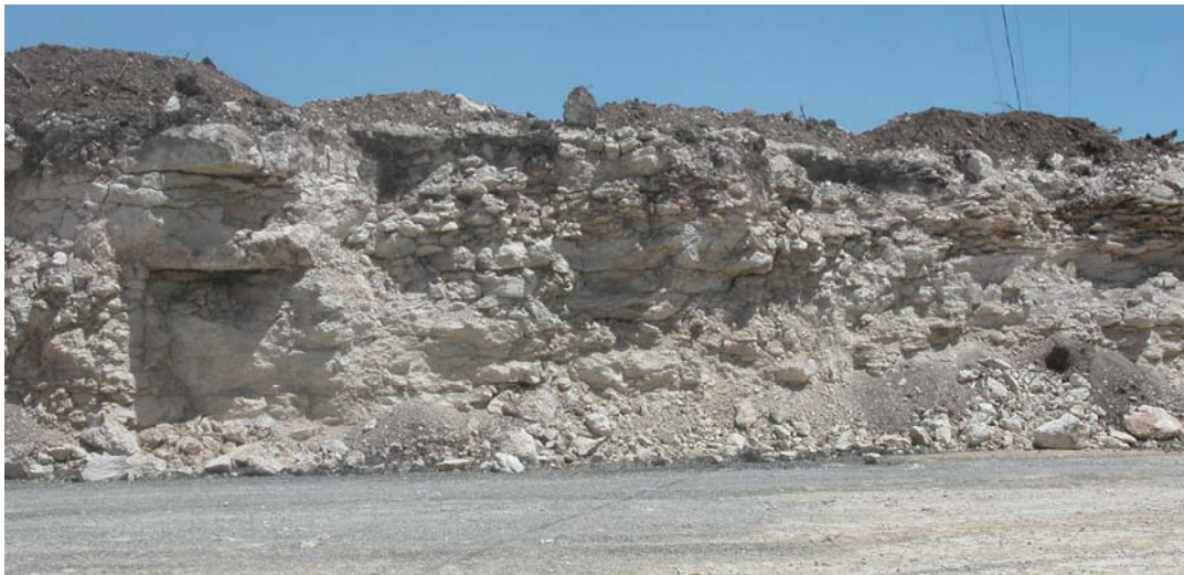
Figure 5. Working Face of the Black Pit Showing Four Different Units That Vary in Quality as an Aggregate.
