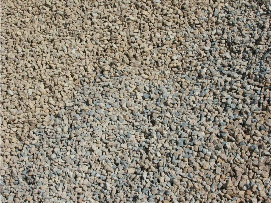
Figure 9. Segregation of Aggregate Types (Gray and Pink) in a Stockpile at the Baird Pit in the Abilene District.
