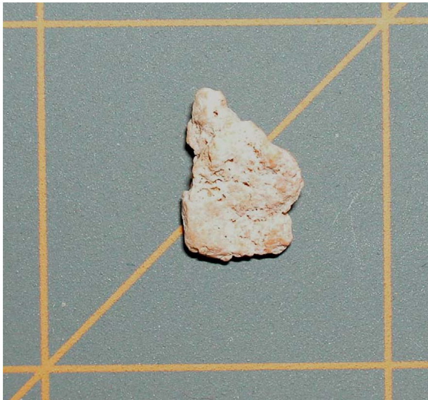
Figure 12. (Top) Thin-Section Photomicrograph Showing Moldic Pores (Blue) in a Limestone Aggregate from the Centex Yearwood Pit. (Bottom) Macroscopic Image of the Same Limestone Aggregate (Note Pits in Surface).
