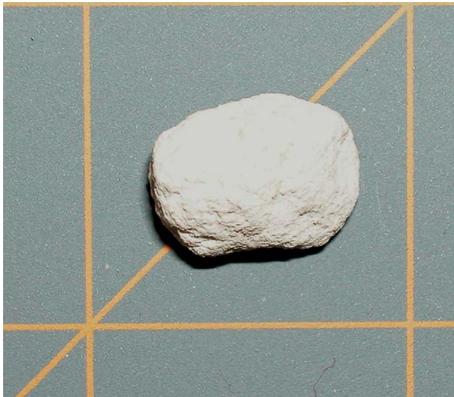
Figure 13. (Top) Thin-Section Photomicrograph Showing Intergranular Pores (Blue) in a Limestone Aggregate from the Centex Yearwood Pit. (Bottom) Macroscopic Image of the Same Limestone Aggregate (Note Roundness).
