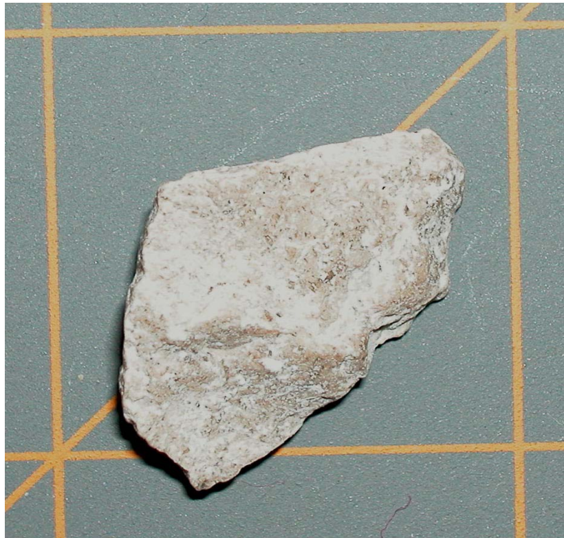
Figure 11. (Top) Thin-Section Photomicrograph of a Limestone Aggregate from the Vulcan Black Pit Showing No Pores. (Bottom) Macroscopic Image of the Same Limestone Aggregate (Note Angularity).
