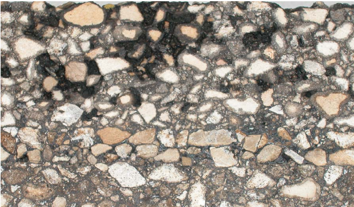
Figure 7. Sample from US-84 in Tyler County Showing Aggregates with a Lot of Absorbed Asphalt.
