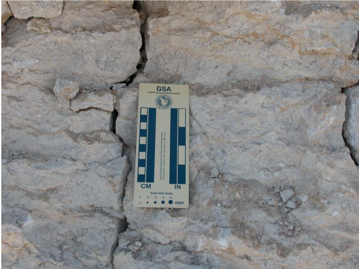
Figure 2. The Semihorizontal Tan Lines in the Top One-Third of the Image are Stylolites from the Black Quarry.
