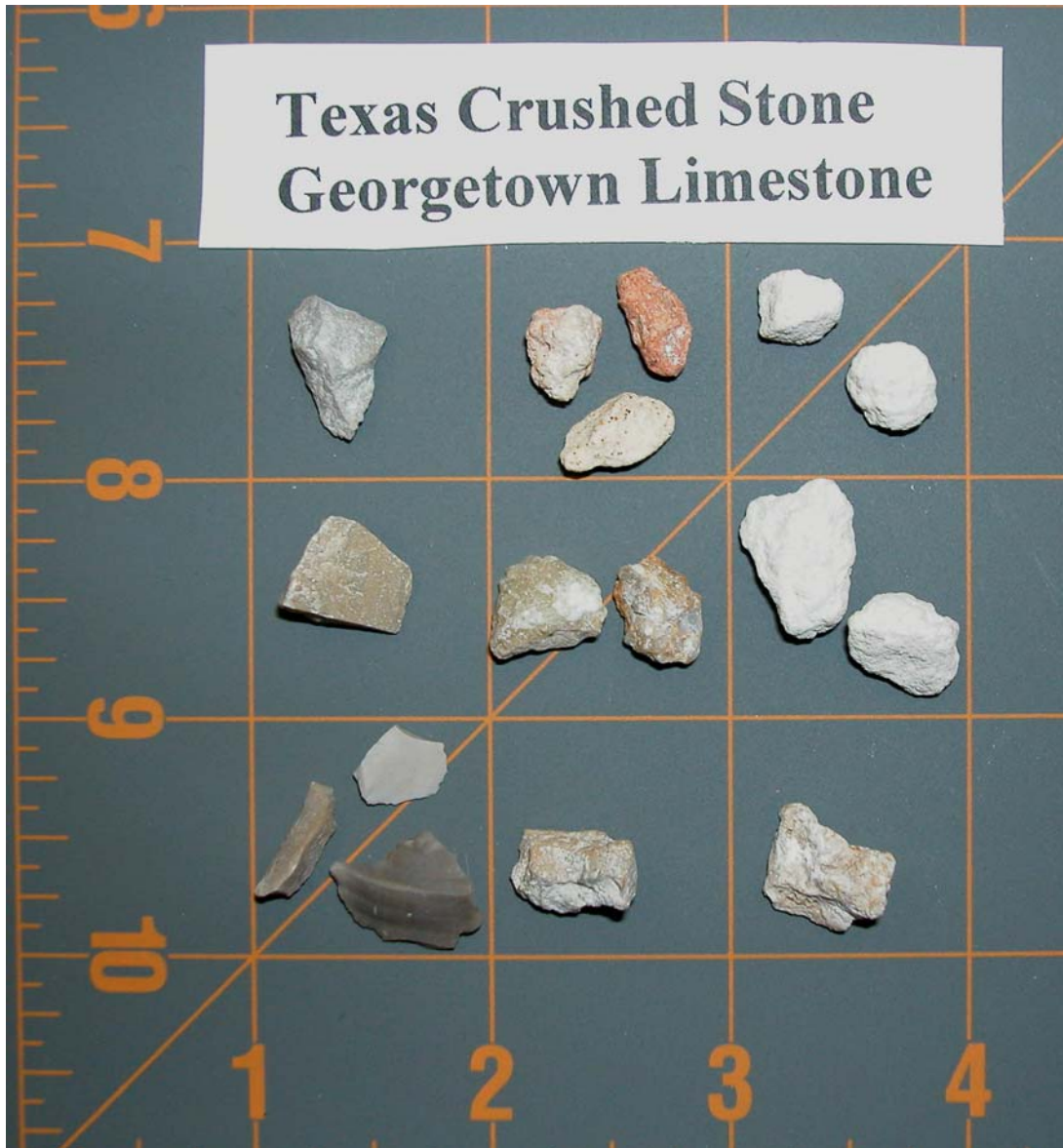
Figure 8. Aggregates from the Same Stockpile Showing Variations in Porosity, Angularity, and Mineralogy.
