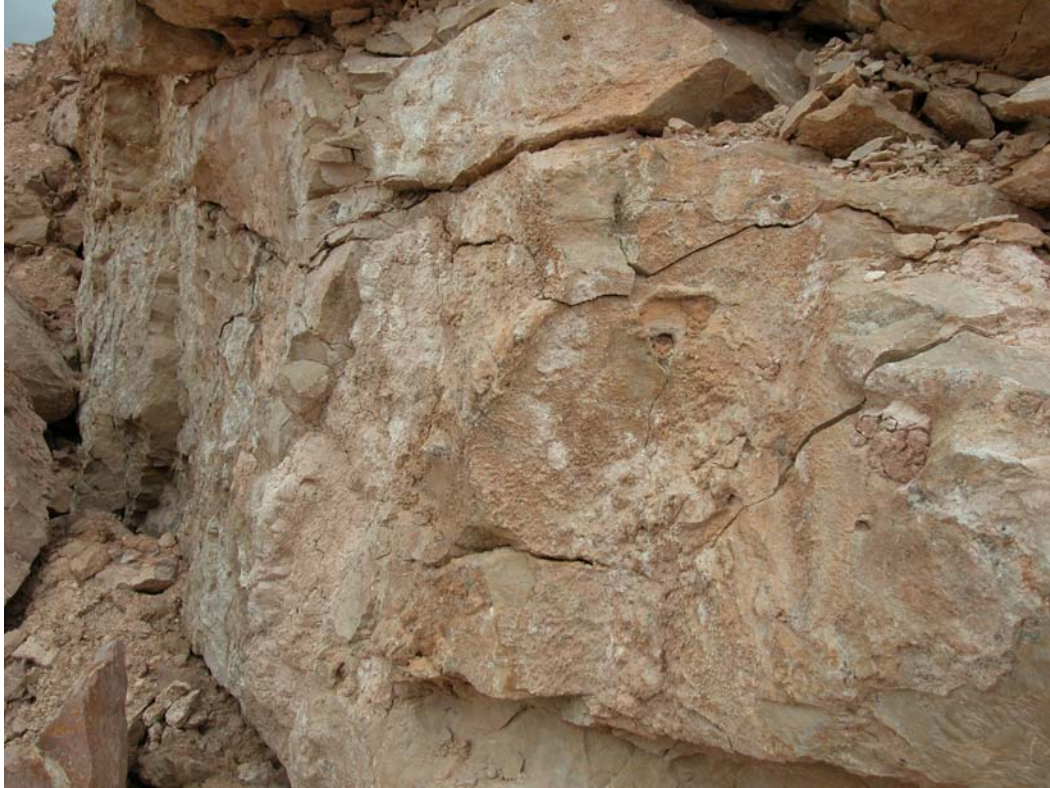
Figure 10. Vertical Fracture at the Price Clements Pit Showing Grayish Orange-Pink Clay Attached to a Pale Yellowish Brown Limestone Block.
