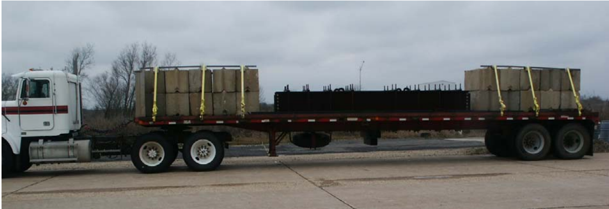
Figure 6.2. Tractor-Trailer Used for Plate Bearing Test.
