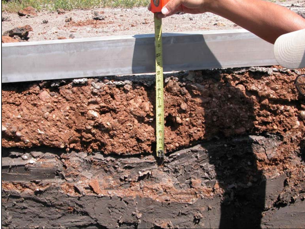
Figure 6.23. View of Pavement Cross-Section at the Uncrushed Gravel Base Trench.
