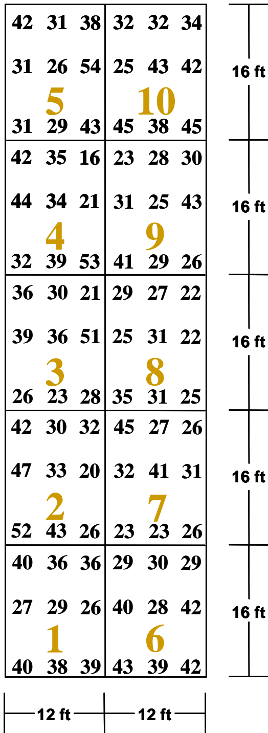
Figure C17. DSPA Test Results on Clay Subgrade Showing Individual DSPA Readings on Flexible Base Section Grid.
