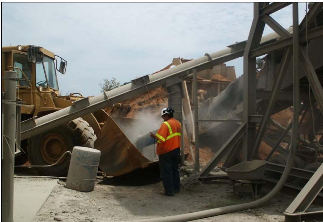
(b) Diverting Cement to Front-End Loader for Weighing.
