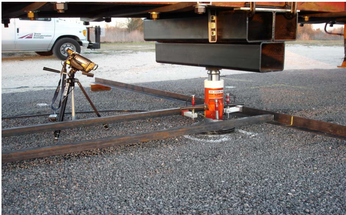
Figure 6.1. Plate Bearing Test Setup.
