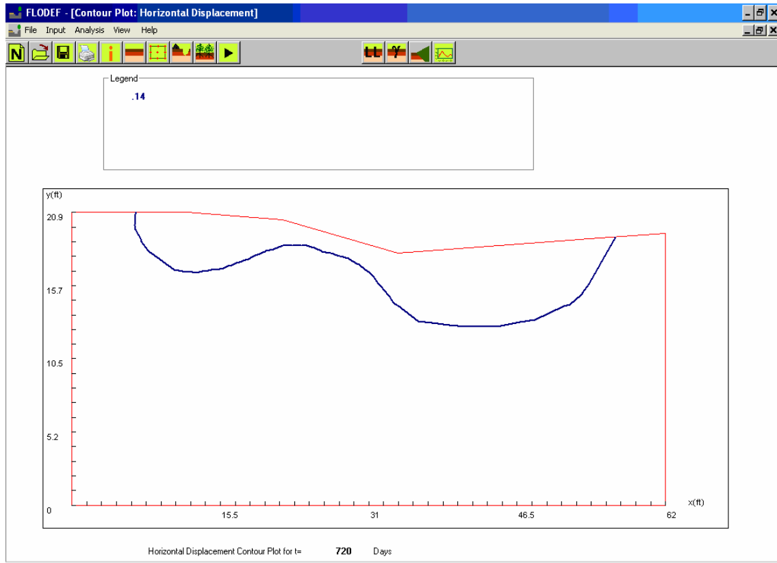
Figure 62. Output Plots Screens: Contour Plots Screens-Horizontal Displacement.
