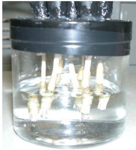
Figure B-2. The Thermocouple Psychrometer Calibration Setup.
