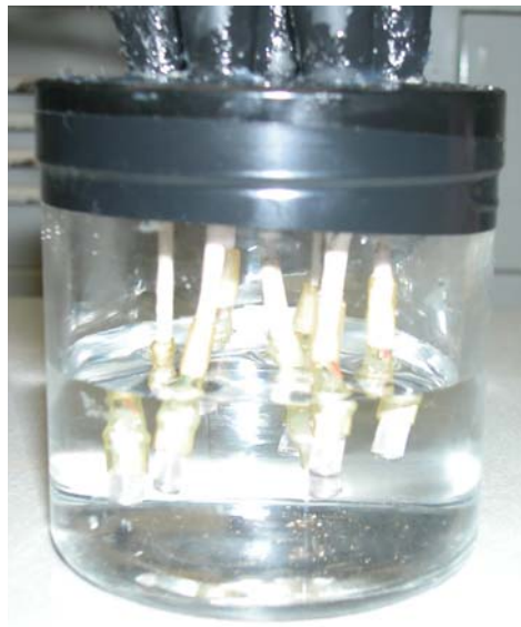
Figure C-2. The Thermocouple Psychrometer Calibration Setup.
