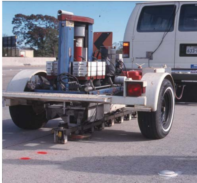
Figure 44. TxDOT's Falling Weight Deflectometer.
