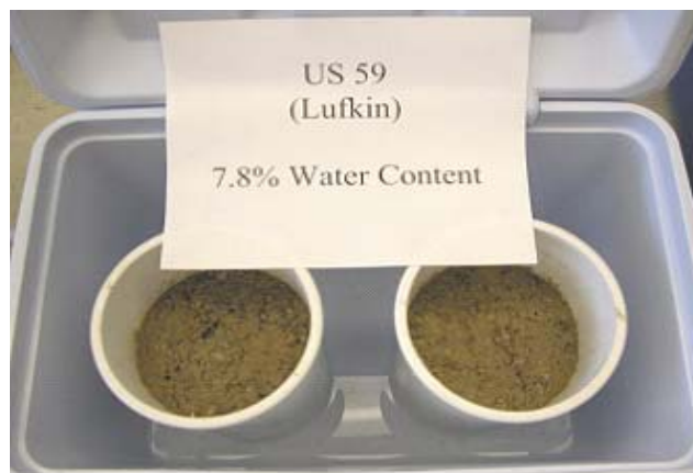
Figure 15. Samples of Base in TST Test.
