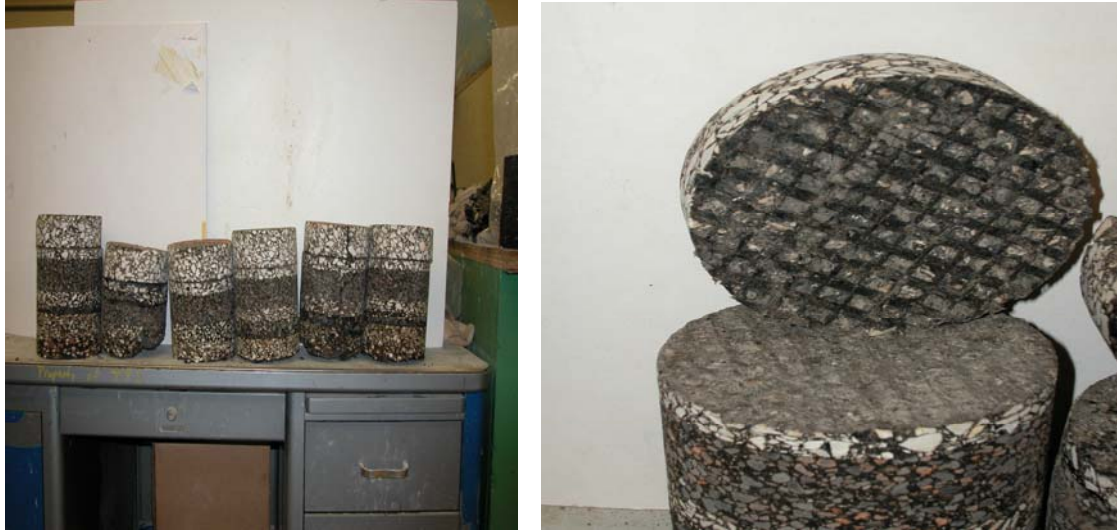
Figure 27. Cores Removed from the Lufkin Section on US 59.
