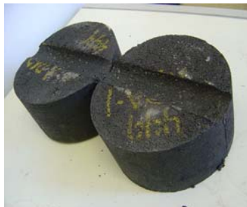
Figure 25. Strata® Samples after 300 Load Repetitions.
