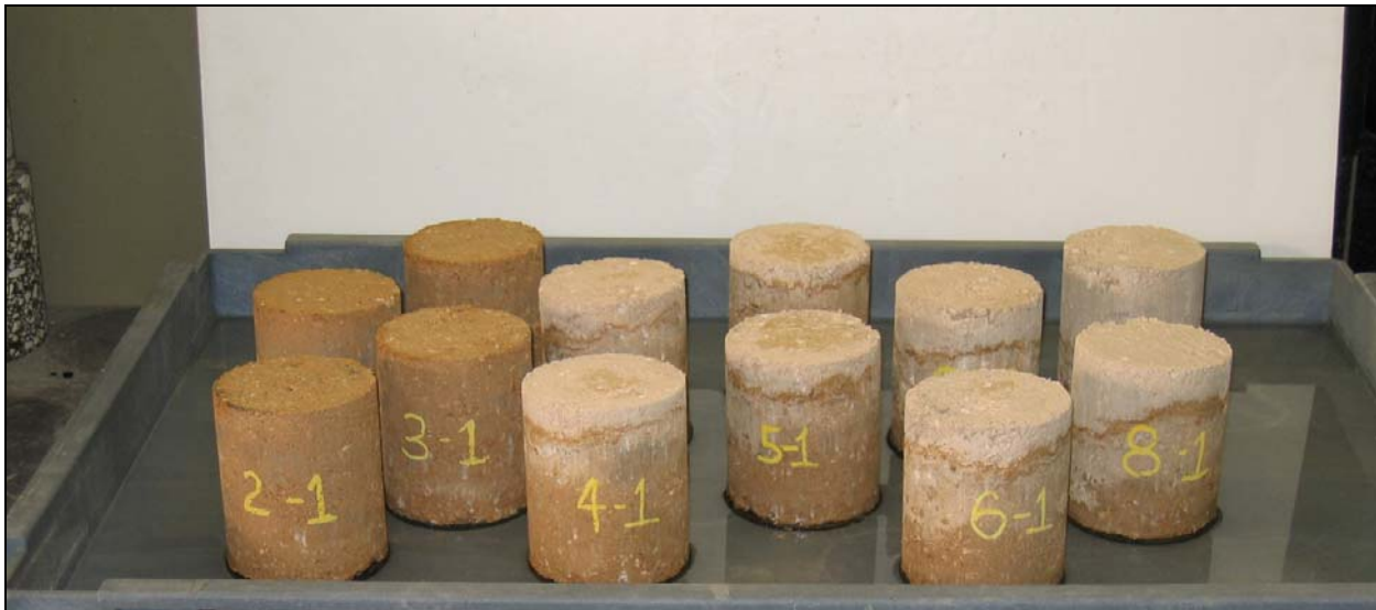
Figure 3.1. Texas Crushed Stone Cement-Treated Base after Tube Suction Test. (l to r: 2, 3, 4, 5, 6, and 8 percent cement)
