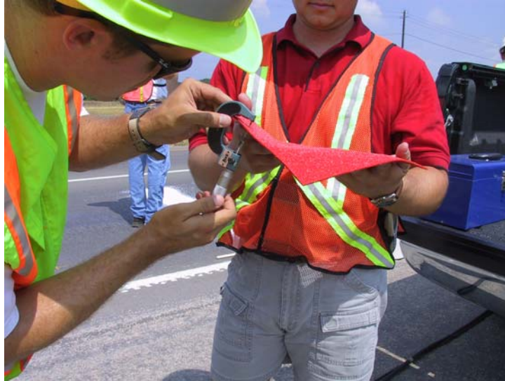
Figure 4. Thickness Measurements on a Piece of Red Preformed Thermoplastic.
