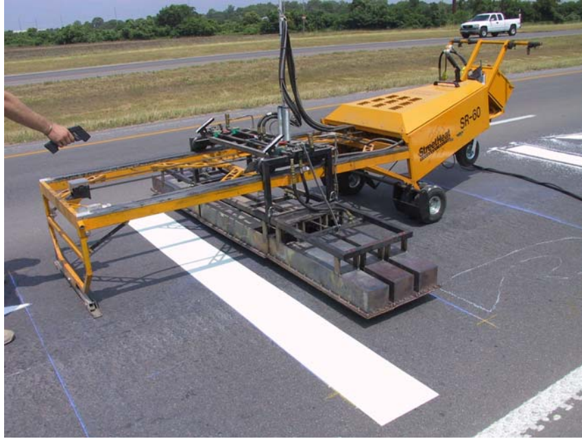
Figure 13. The Streetprint Melting a Transverse Line.
