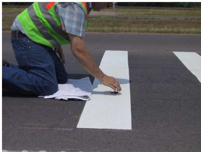
Figure 5. Bead Embedment Inspection Using a Jeweler's Loupe.
