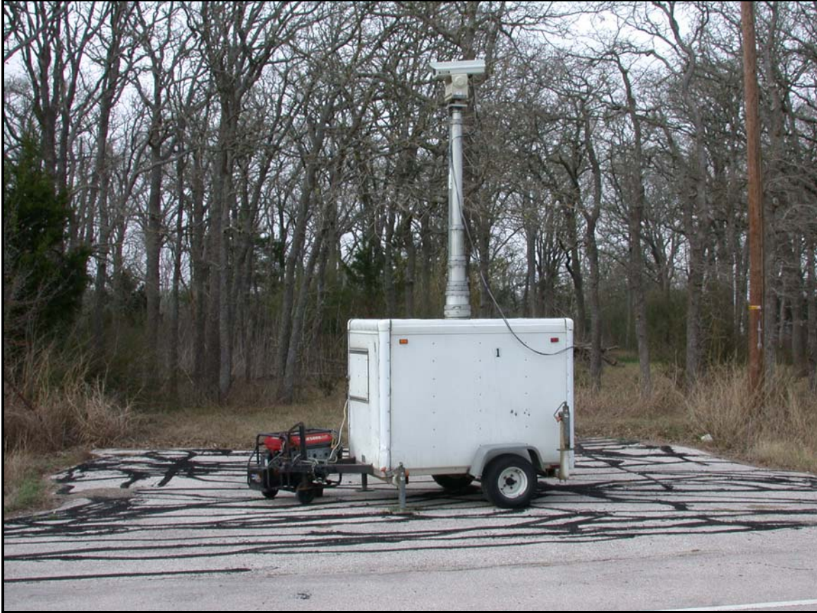
Figure 19. Video Camera Trailer Used for Lane Choice Data Collection.
