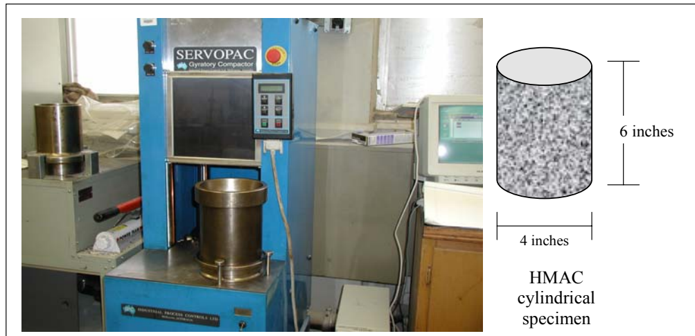
Figure 2-2. Standard SGC Compactor and HMAC Cylindrical Test Specimen.
