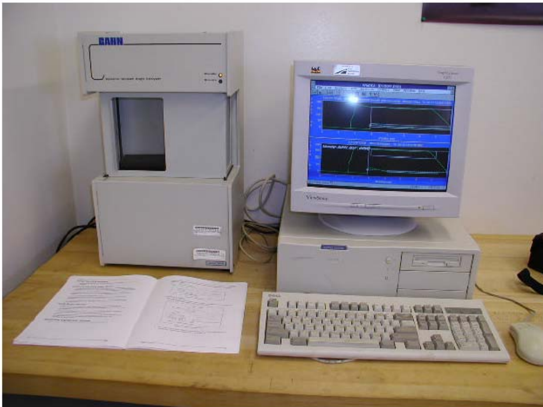
Figure 5-11. The DCA Force Balance and Computer Setup - Wilhelmy Plate Test.
