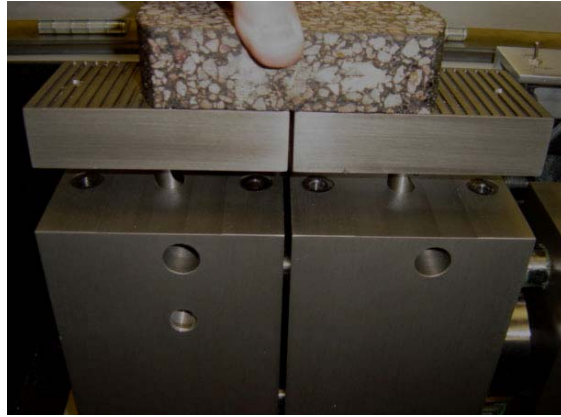
Figure 8. Insert Pins into Machine Making Sure Cutout on Center Pin Is on the Side Facing the Cams (Cutout Facing to Right).
