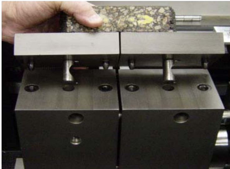
Figure 7. Position Right Hand Block with Left/Right Switch to Line Up Pins on Test Specimen Assembly.
