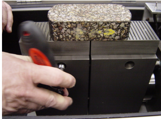
Figure 9. Tighten Cam until It Locks in Place.
