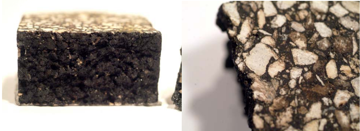
Figure 15. Specimen with Absorptive Limestone.
