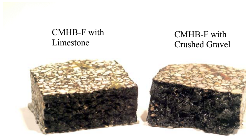
Figure 28. Crack Surfaces of Broken Specimens.
