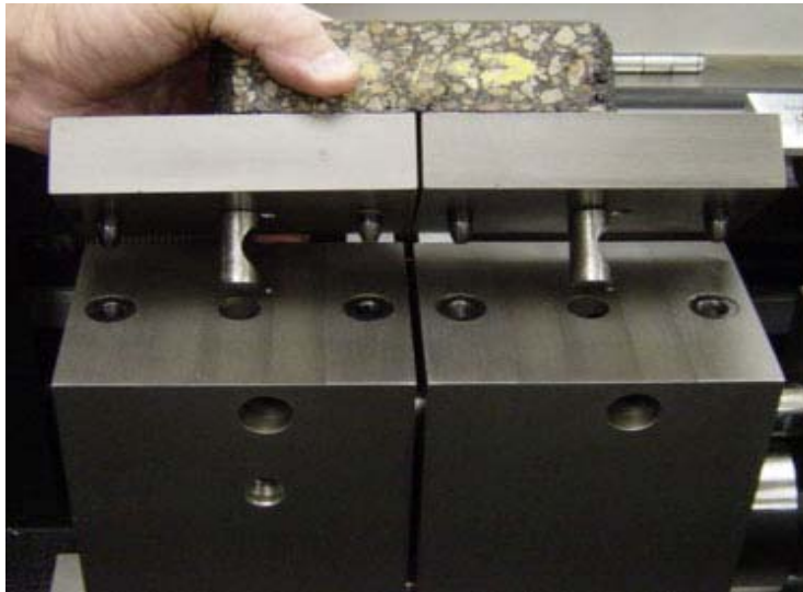
Figure 52. Position Right Hand Block with Left/Right Switch to Line Up Pins on Test Specimen Assembly.
