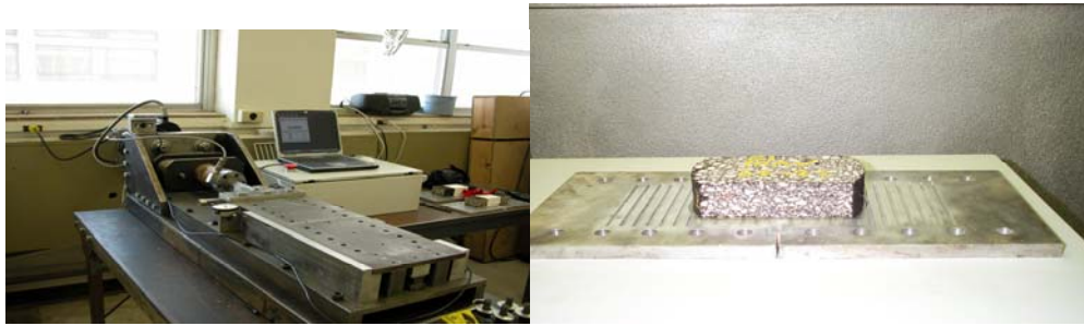
Figure 40. TTI's Existing Overlay Tester.
