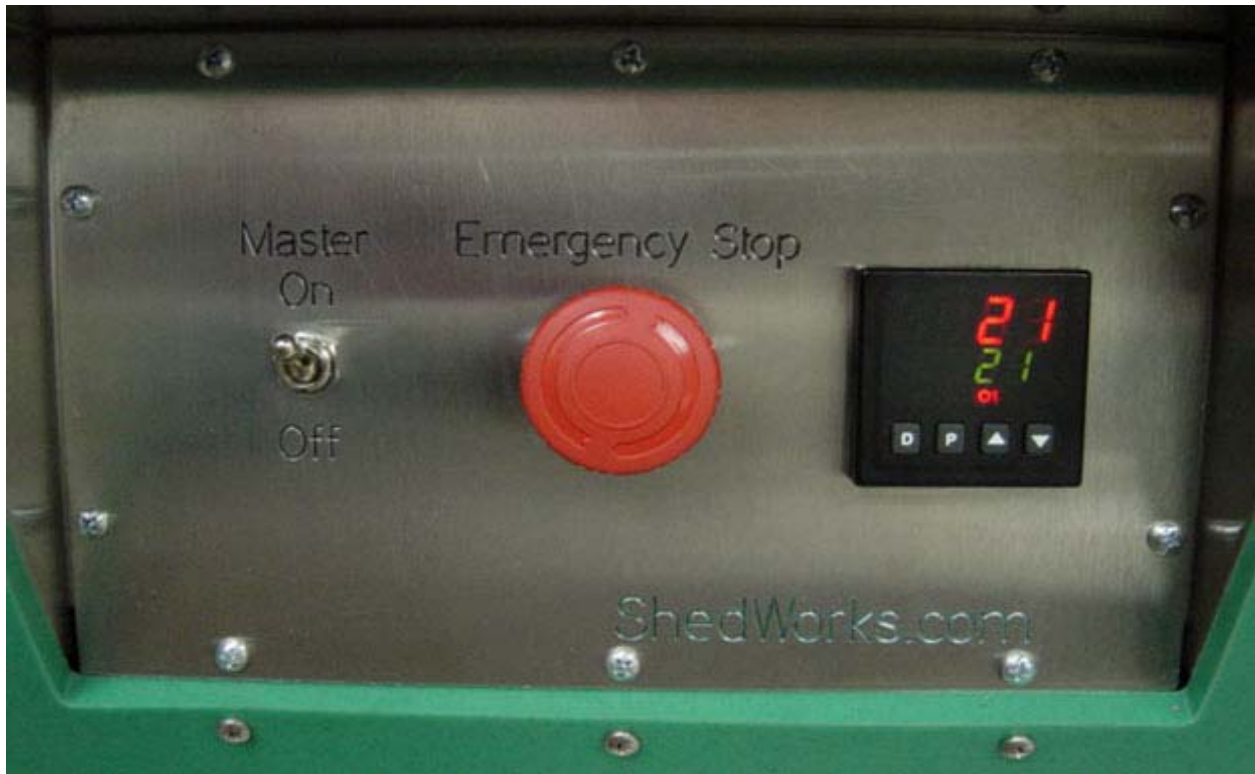
Figure 49. Main Control Panel.
