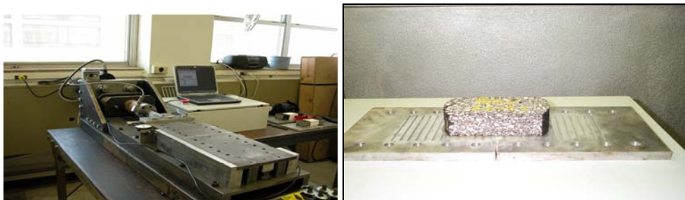
Figure 3. Upgraded TTI Overlay Tester Equipment, Plate, and Specimen.
