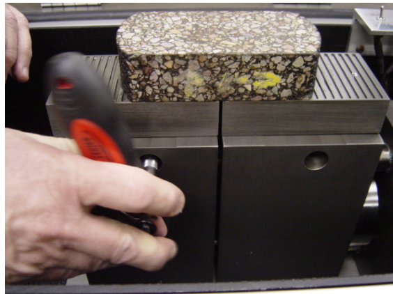
Figure 54. Tighten Cam until it Locks in Place.
