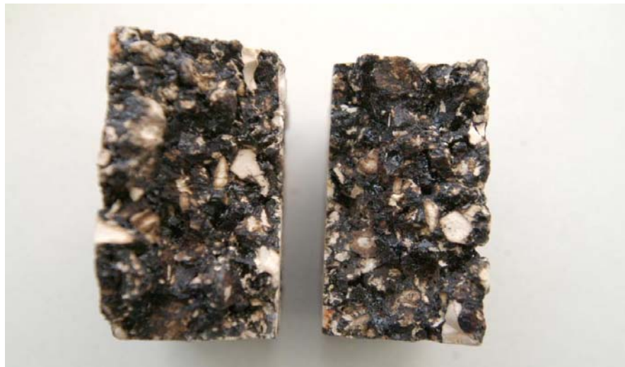
(c) Crack through Aggregate
