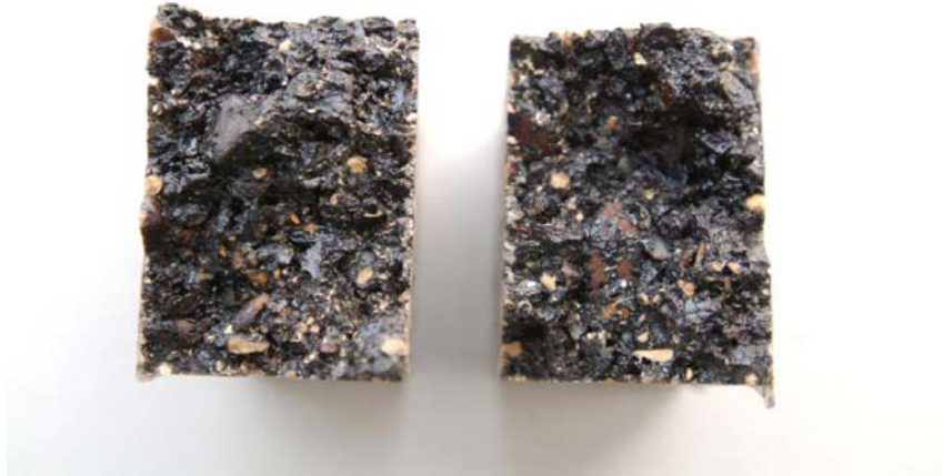
(b) Crack through Interface
