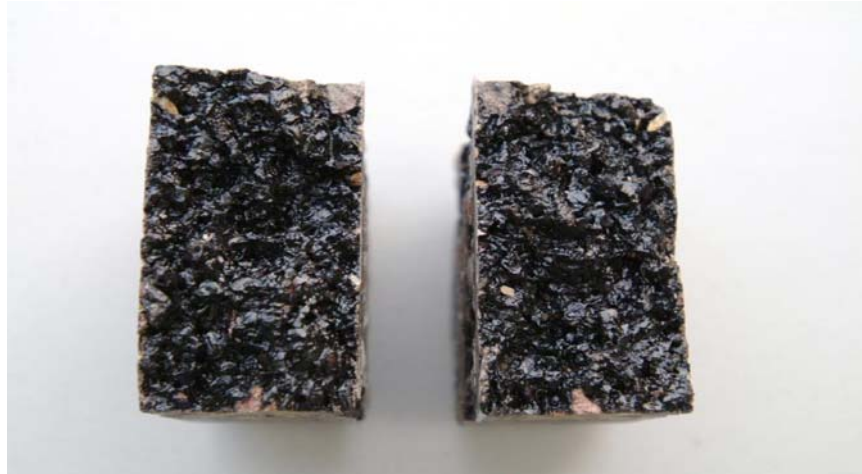
(a) Crack through Binder
