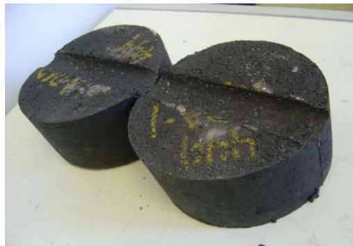
Figure 23. Strata Material Rut Depth after Asphalt Pavement Analyzer Test (more than 8 mm after 2500 Load Repetitions at 64 °C and Loading Pressure of 100 psi).
