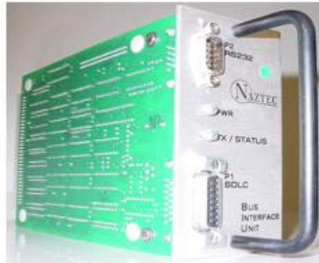
Figure 7. Enhanced Bus Interface Unit (BIU) Used with TS-2 Implementations of TSPMS.
