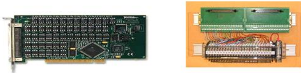
Figure 5. National Instruments PCI 6527 Digital I/O Card and a Terminal Strip Used with TS-1 Implementations of TSPMS.
