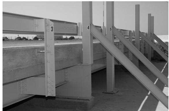
**Figure 24. Llano Truss Bridge Installation before Test 444193-1.**
