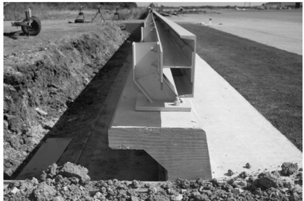
**Figure 36. U.S. 281 Truss Bridge Installation before Test 444193-2.**
