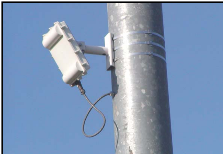
Figure 3-5. SmartSensor by Wavetronix Detection Used on Spur 408.
