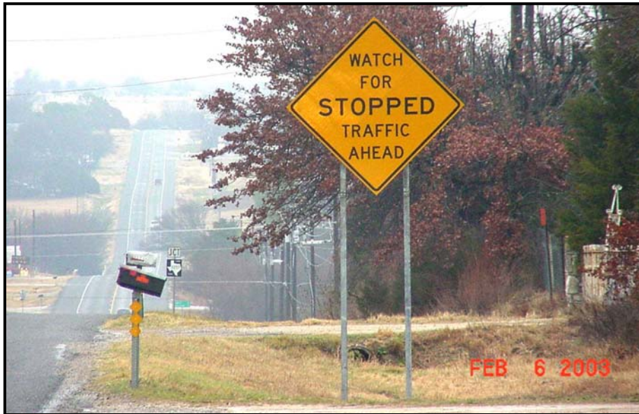
Figure 4-13. Example of Diamond-Shaped Warning Sign – Fort Worth, Texas.
