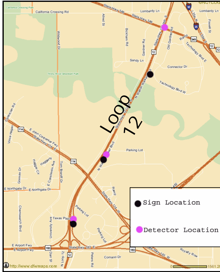
Figure 2-13. Loop 12 Field Test Sign and Detector Locations.
