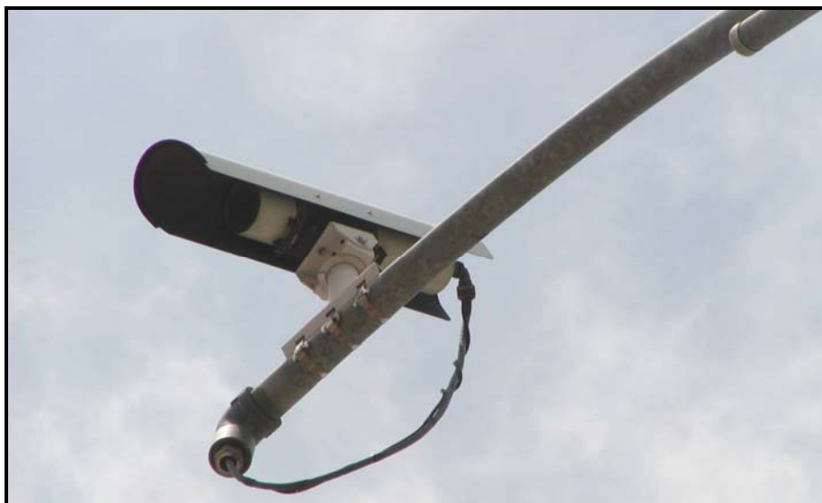
Figure 3-6. Autoscope Video Detection Used on Loop 12.
