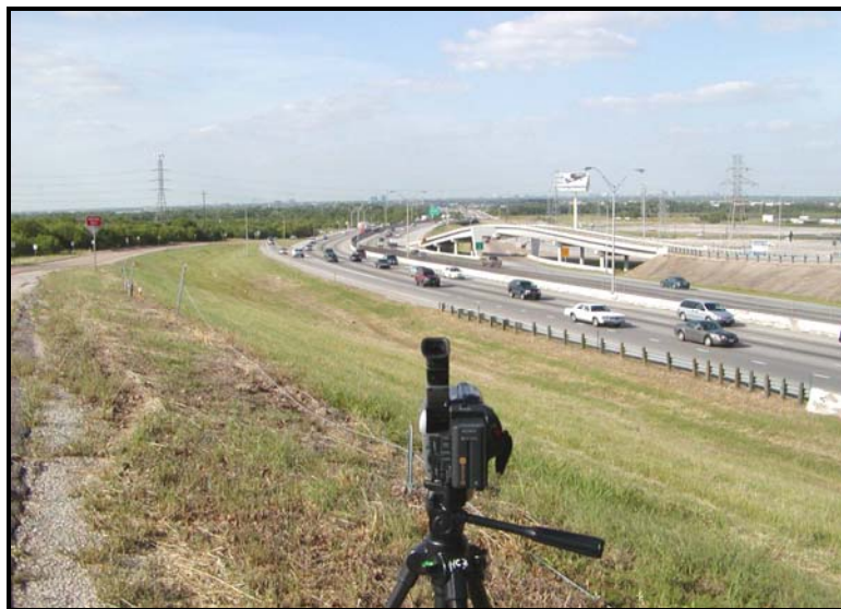
Figure 3-2. Video Tape Data Collection on Loop 12 (Observing Vehicles Moving Away from Camera).
