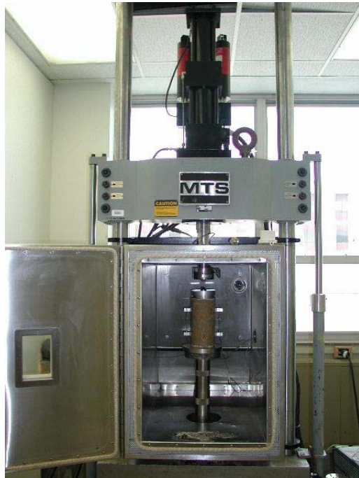
Figure 26. Resilient Modulus Test Setup.
