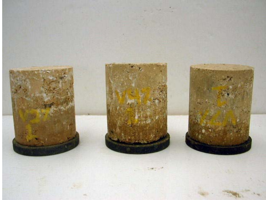
Figure 35. Representative Vulcan Cement-Treated Base after the TST. L to R: 2 percent, 4 percent, and 7 percent Type 1 Cement.
