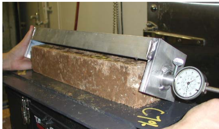
Figure 28. Shrinkage Measurement in Progress.
