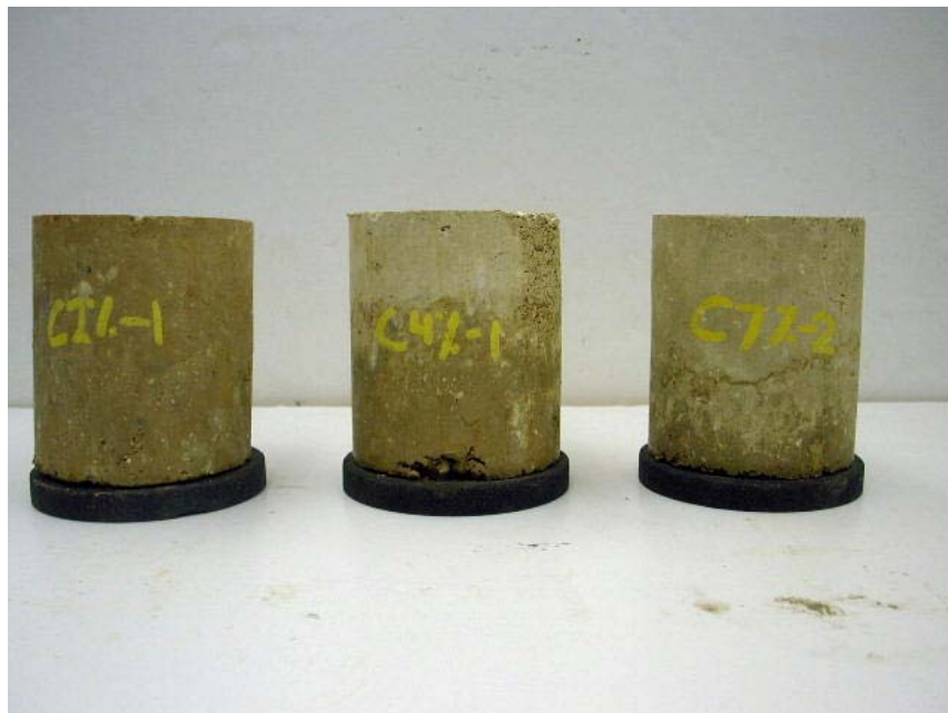
Figure 34. Representative Colorado Cement-Treated Base after the TST. L to R: 2 percent, 4 percent, and 7 percent Type 1 Cement.
