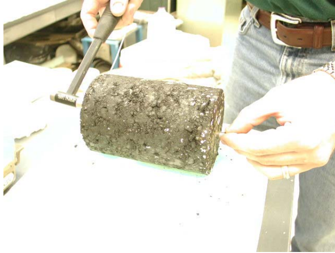
Figure 31. Black Base Specimen Tested for Seismic Modulus.
