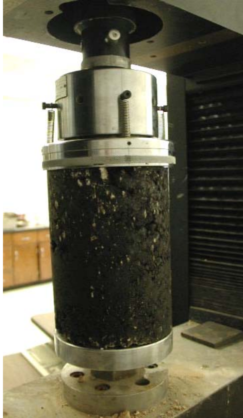
Figure 30. Black Base Specimen in Compression Test.
