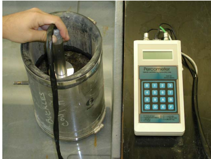
Figure 23. Surface Dielectric Measurements during Tube Suction Test.
