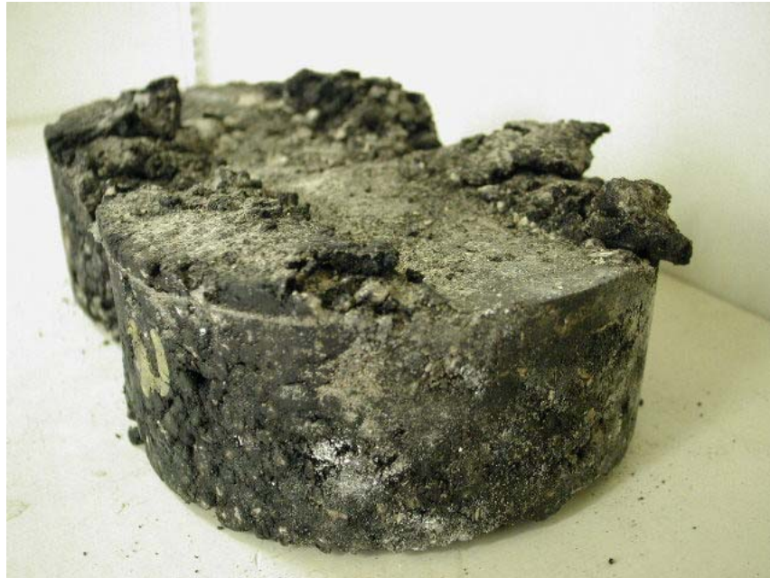
Figure 39. Black Base after Hamburg Test.
