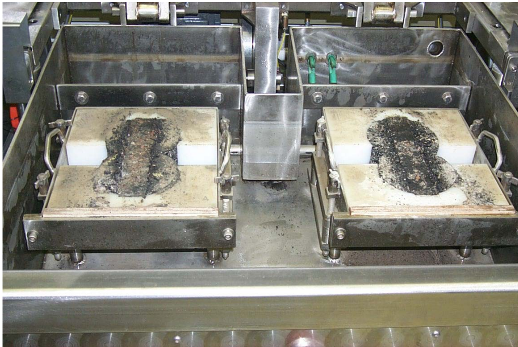
Figure 2-1. Hamburg Wheel Tracking Test.
