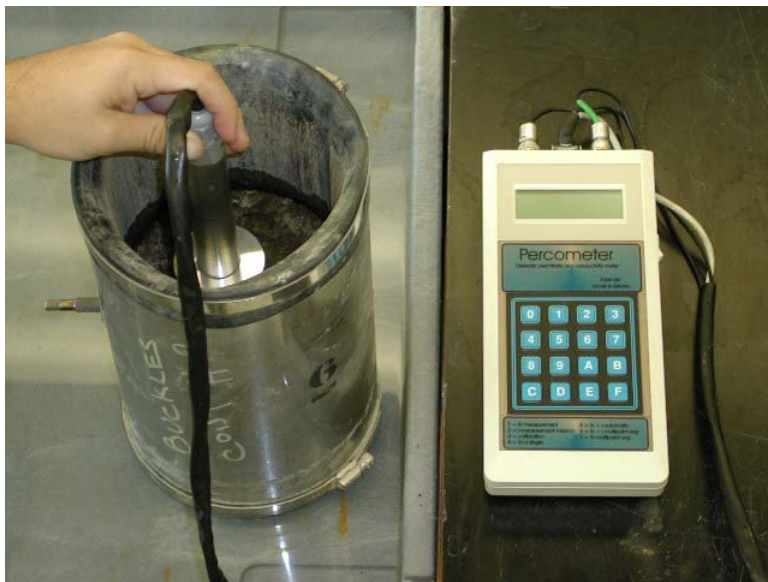
Figure 3-2. Using the Adek Percometer™.
