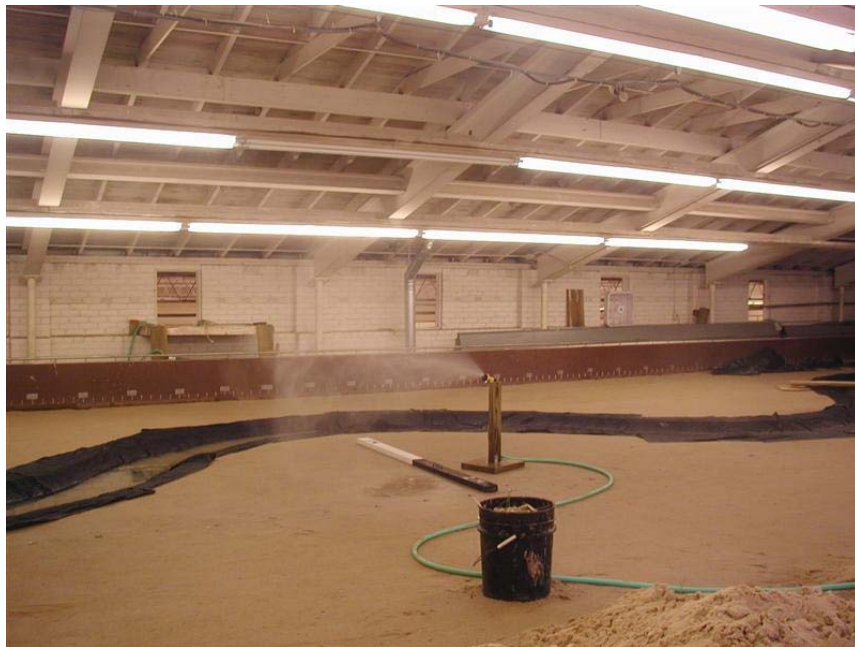
Figure B.8. Sprinkling the Clay Banks.
