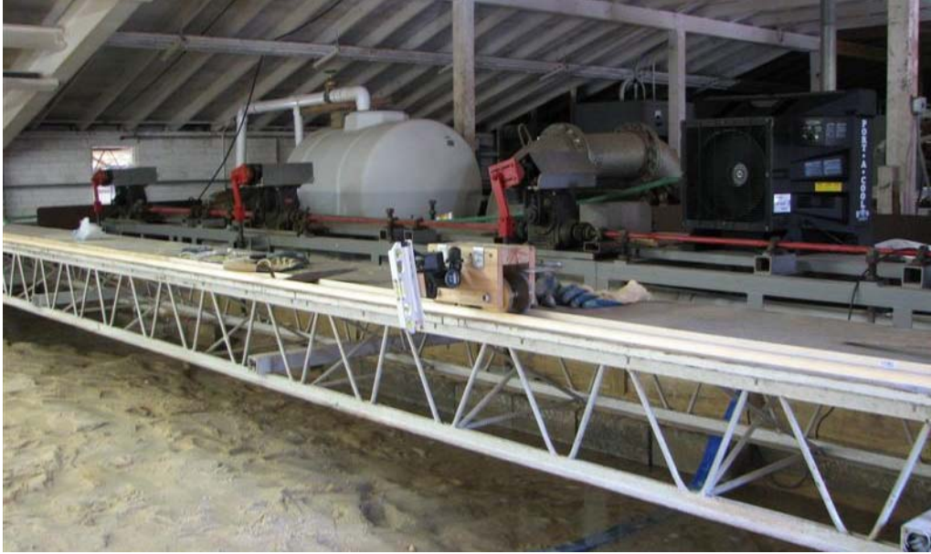
Figure 6.5. Carrier with Laser Sliding on the Bridge for Transverse Coordinate ( y -direction) Measurement.
