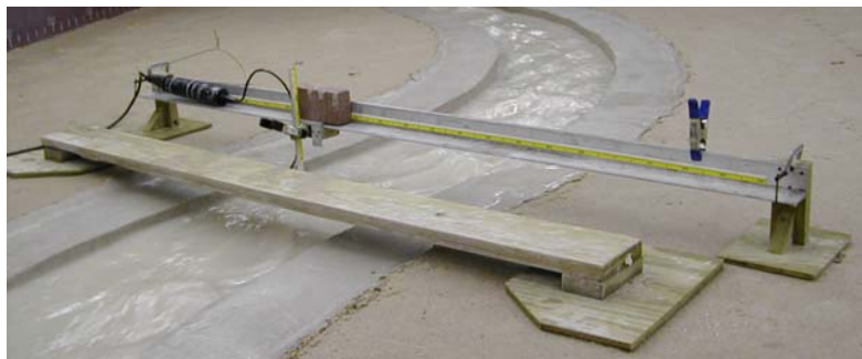
(a) Installed ADV probe on Frame
