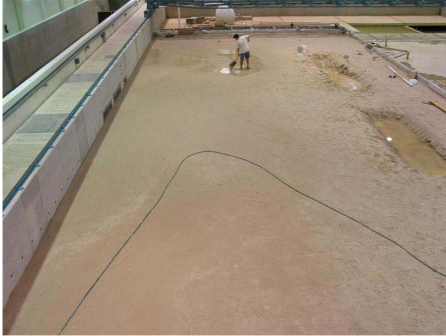
Figure A.1. Filling Sand into the Previous Channel for Next Test.
