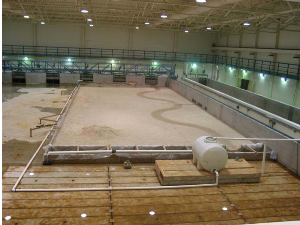
Figure 5. Water Basin and Flume Test Setup in Sand Test.
