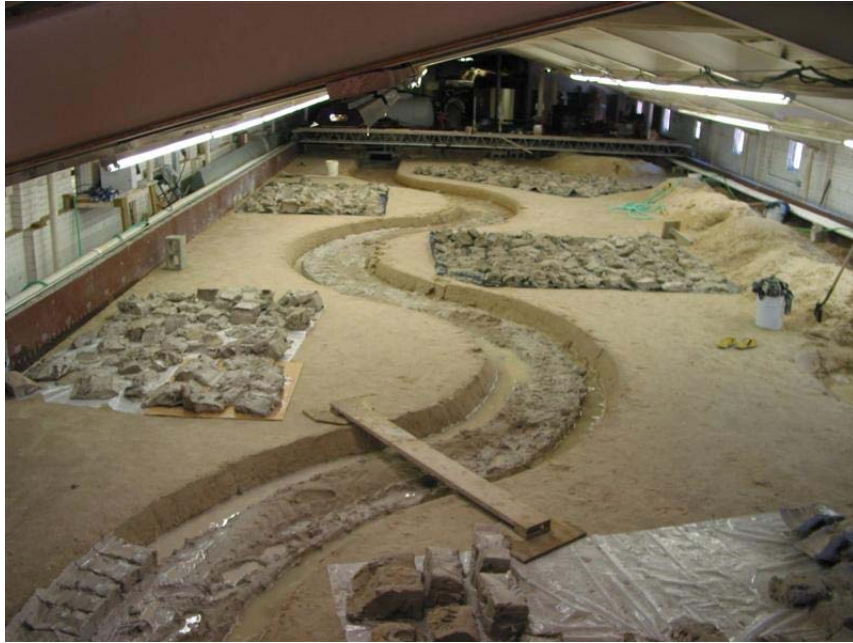
Figure B.1. Retrieving Clay from the Previous Test.
