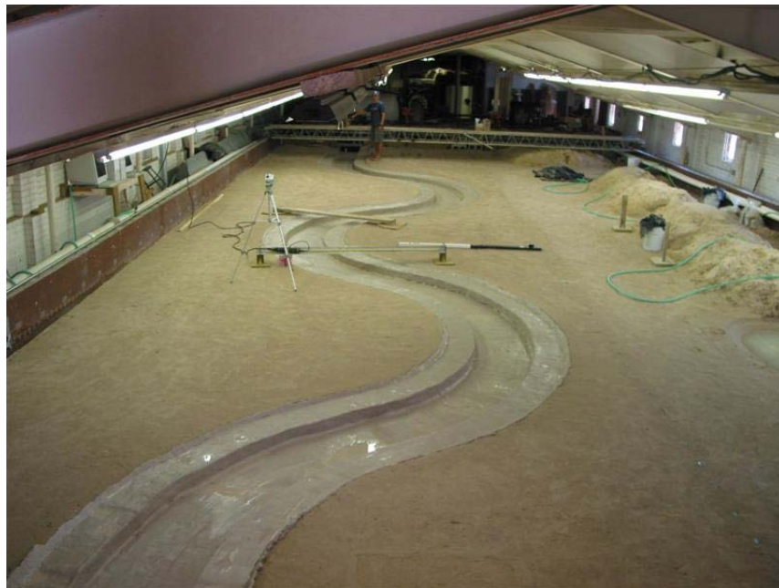
Figure B.12. Initial Condition of Clay Test Case 02 ( R/W = 4 , \phi = 120^\circ , Fr = 0.50 ).
