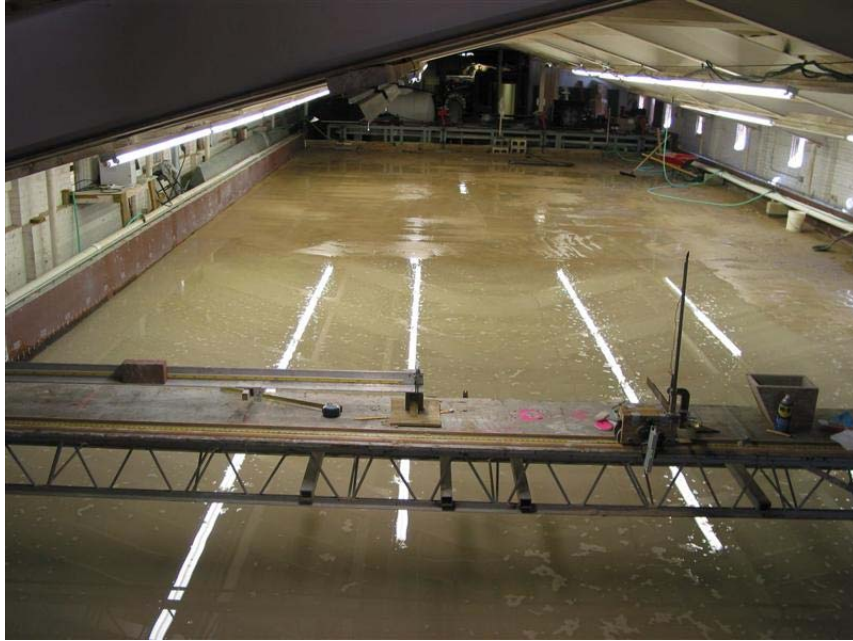
Figure B.3. Leveling the Sand Bed.
