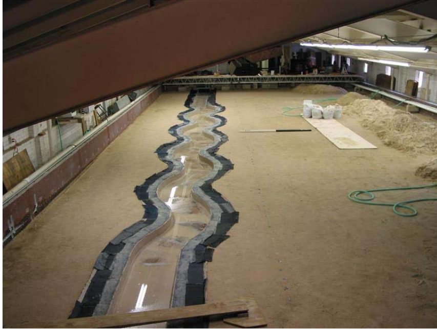
Figure B.20. Initial Condition of Clay Test Case 06 ( R/W = 2 , \phi = 65^\circ , Fr = 0.50 ).
