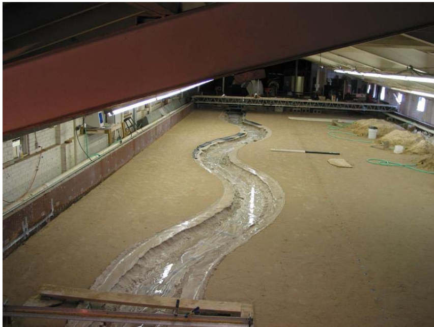
Figure B.15. Final Condition of Clay Test Case 03 ( t = 163.5 hr).
