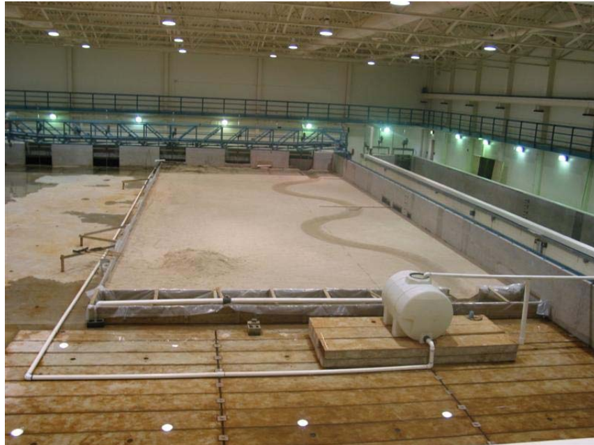
Figure 5.1. Water Basin and Flume Test Setup.
