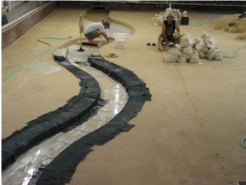
Figure B.7. Placing the Clay Banks and Covering with Wet Cloth.
