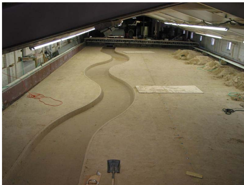
Figure B.6. Digging the Sand Channel.
