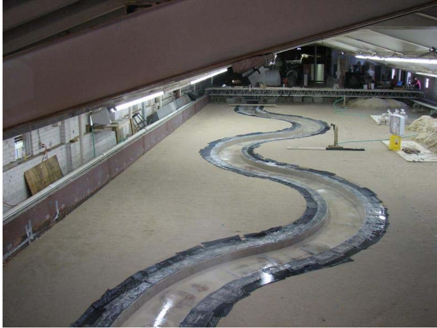
Figure B.22. Initial Condition of Clay Test Case 07 ( R/W = 4 , \phi = 120^\circ , Fr = 0.50 ).
