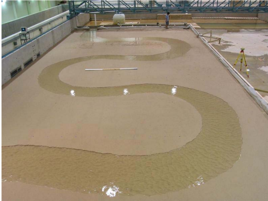
Figure A.11. 147 hr Plan Form of Sand Test Case 08 ( R/W = 4 , \phi = 220^\circ , Fr = 0.30 ).
