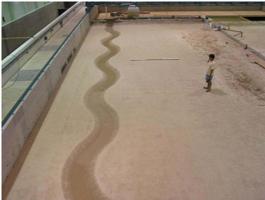
Figure A.6. Channel Initial Geometry with Water.
