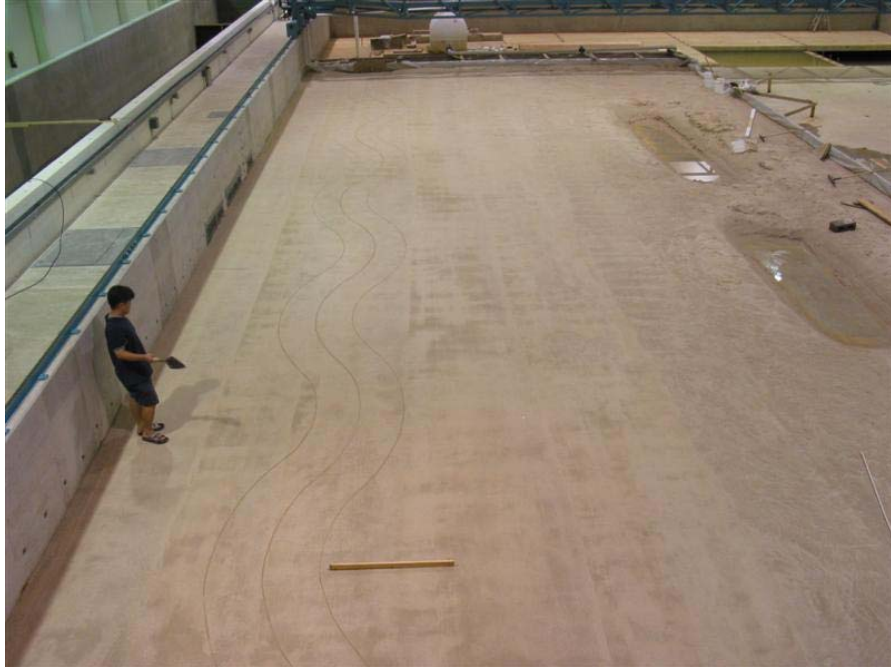
Figure A.3. Sketching Channel Contour on the Sand Bed.
