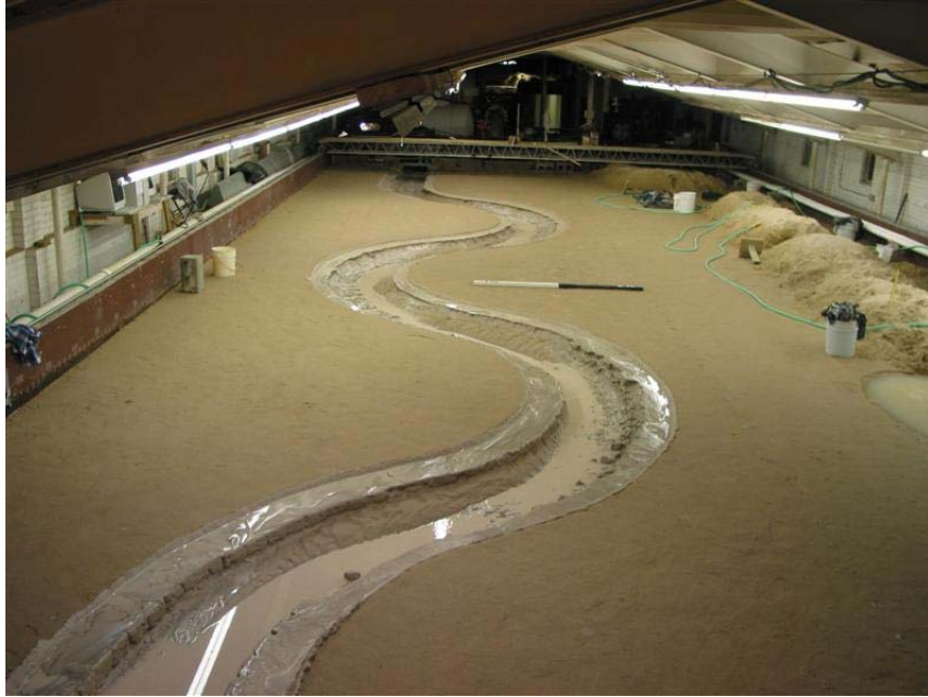
Figure B.13. Final Condition of Clay Test Case 02 ( t = 106.5 hr).
