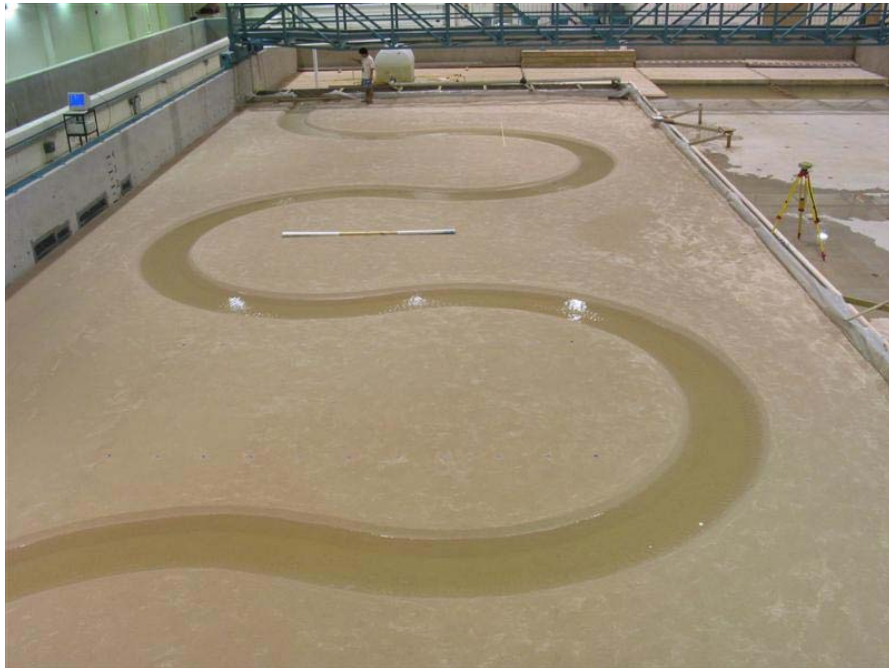
Figure A.10. Initial Plan Form of Sand Test Case 08 ( R/W = 4 , \phi = 220^\circ , Fr = 0.30 ).
