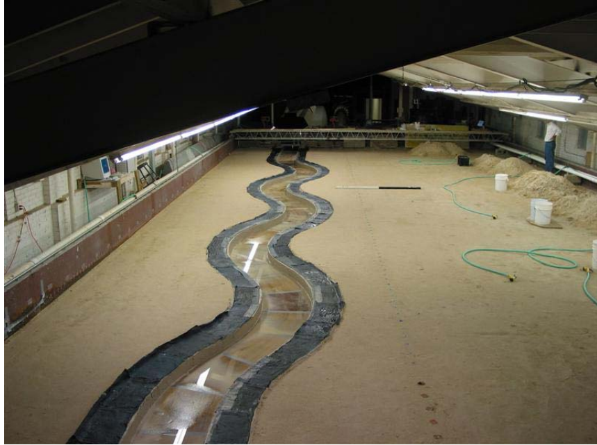
Figure B.16. Initial Condition of Clay Test Case 04 ( R/W = 4 , \phi = 65^\circ , Fr = 0.50 ).
