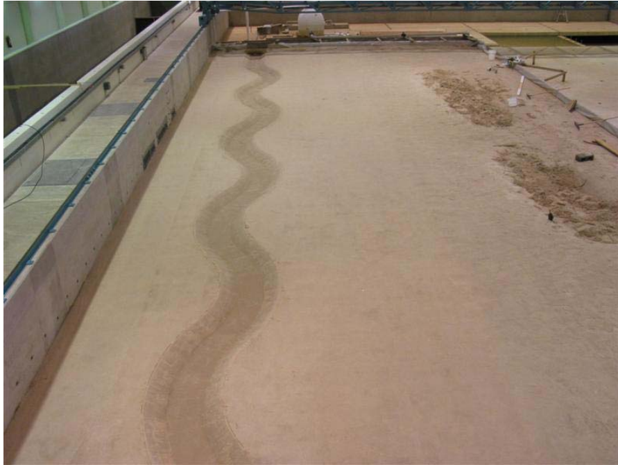
Figure A.5. Completion of the Sand Channel.
