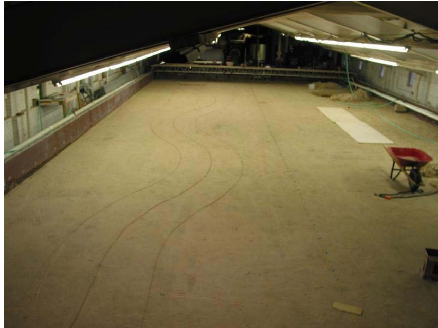
Figure B.5. Drawing the Contour of the Sand Channel.
