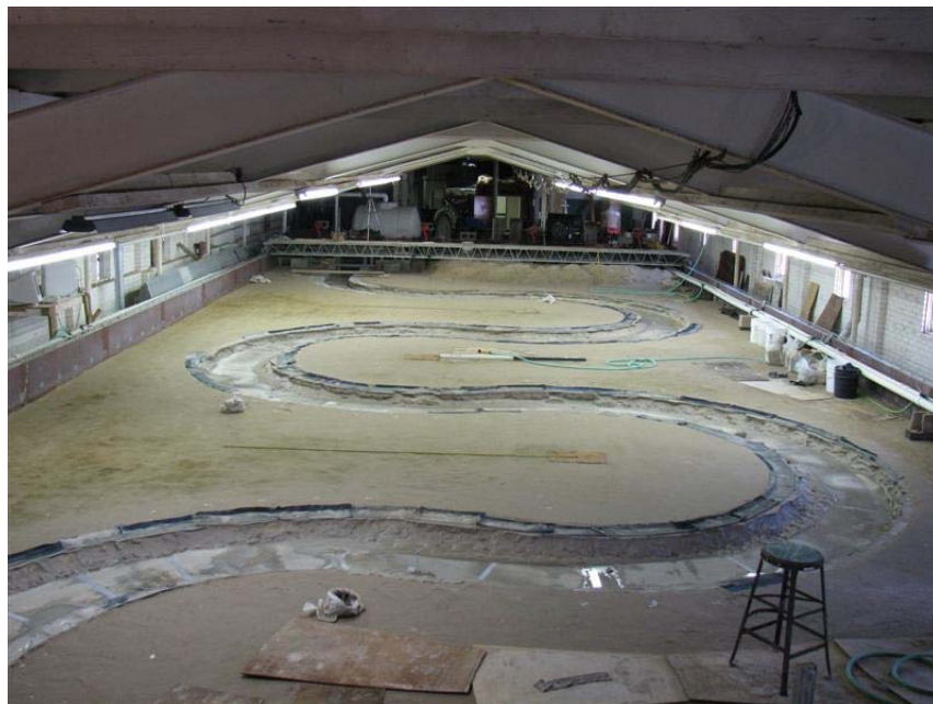
Figure B.25. Final Condition of Clay Test Case 08 ( t = 336 hr).
