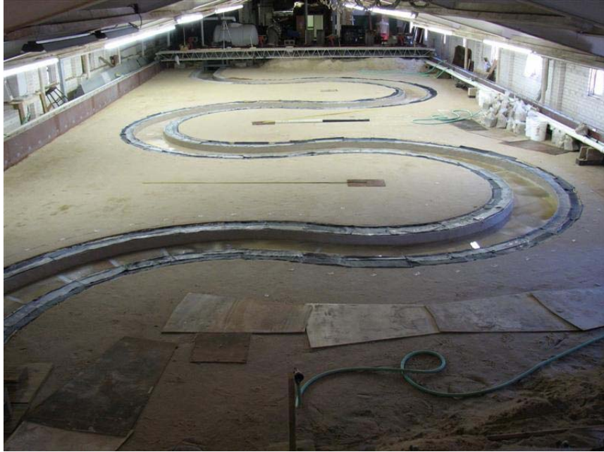
Figure B.9. Completion of the Clay Channel.
