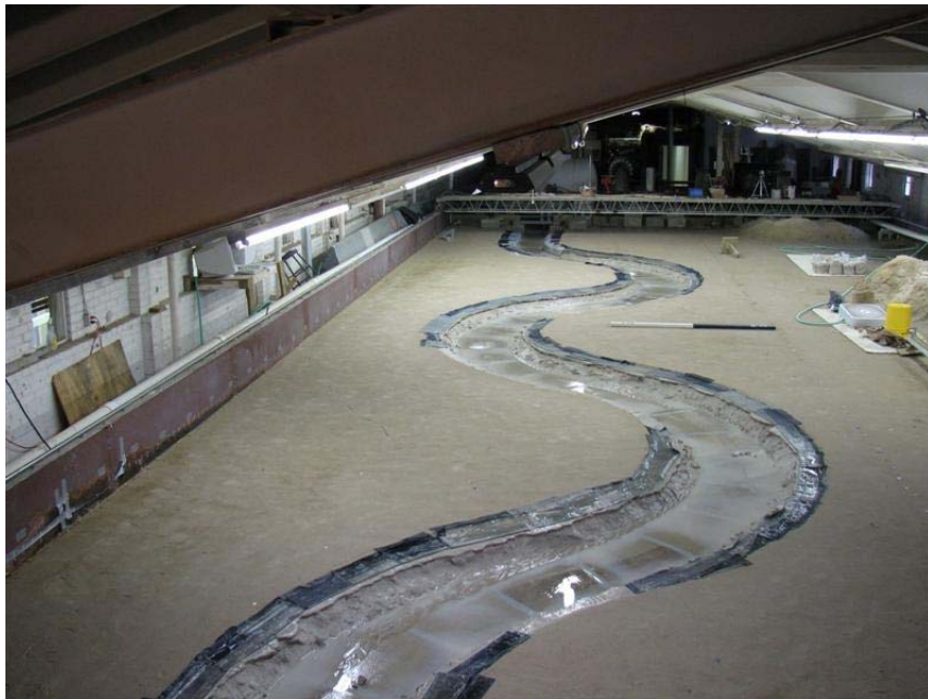
Figure B.23. Final Condition of Clay Test Case 07 ( t = 192 hr).
