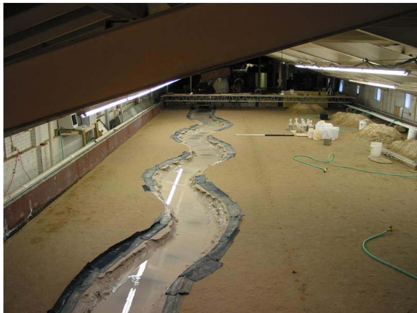
Figure B.17. Final Condition of Clay Test Case 04 ( t = 268 hr).
