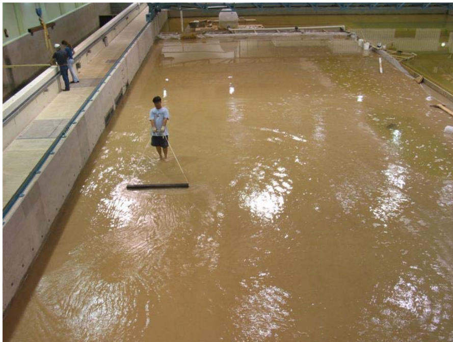
Figure A.2. Leveling Sand Bed.
