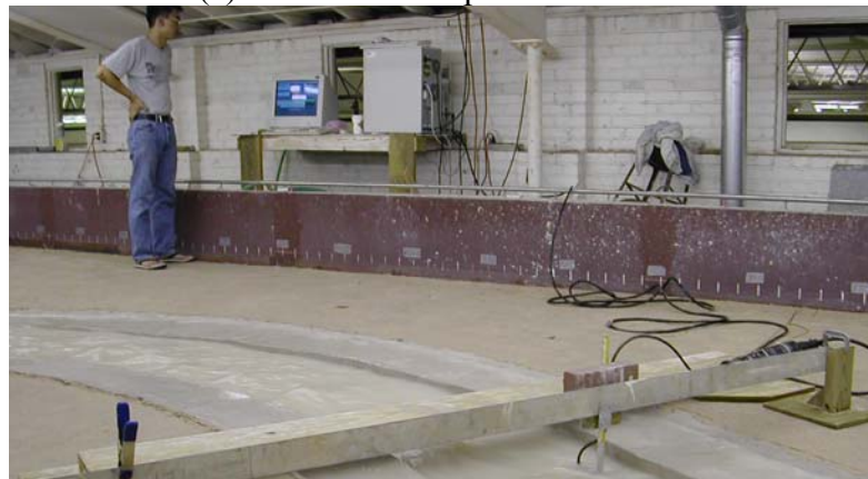
(b) Data Acquisition Computer Connected to ADV probe
