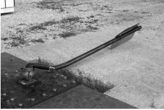
Figure 2-3: Schedule 10 Triangular slip base that did not perform as intended.
