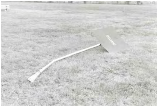
Figure 2-9: Schedule 10 socket system that performed as intended
