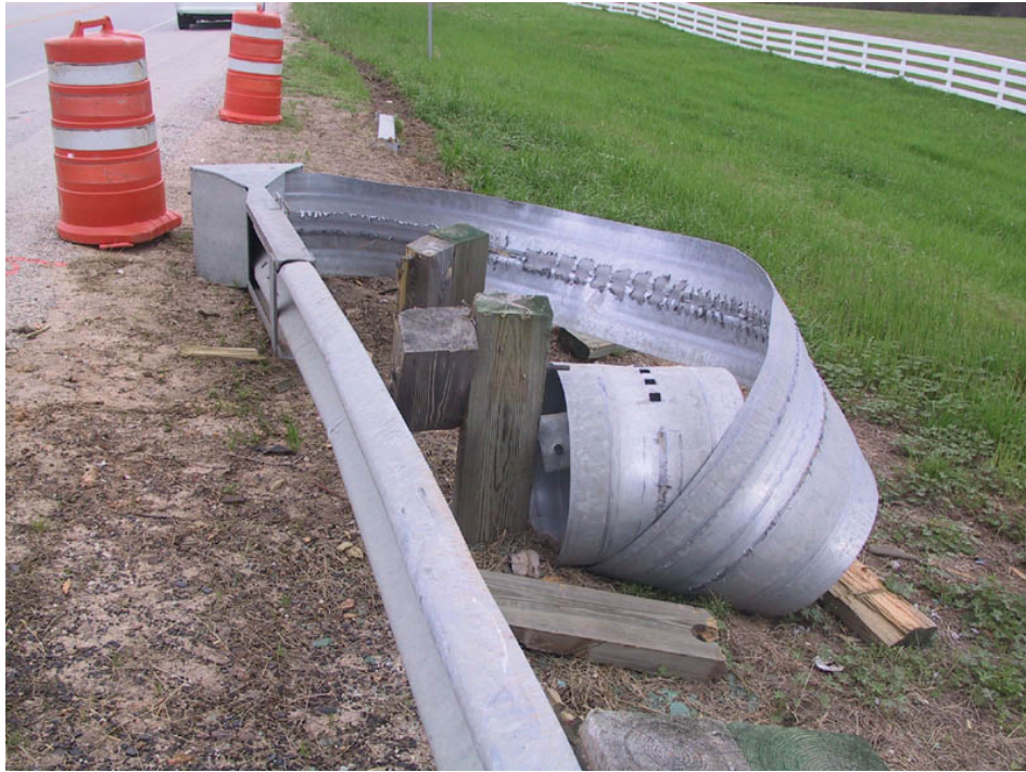
Figure D1: A Photograph Taken During the Pilot Test of an ET-2000 SGT That Performed As Intended.
