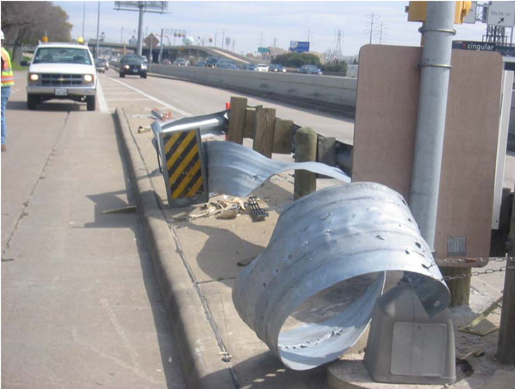
Figure D5: An Example of An Extruder Head Buckling: Note that, In This Case, The SGT Performed As Intended. The Buckling of the Extruder Head Do Not In Itself Imply That the Device Did Not Perform As Intended.
