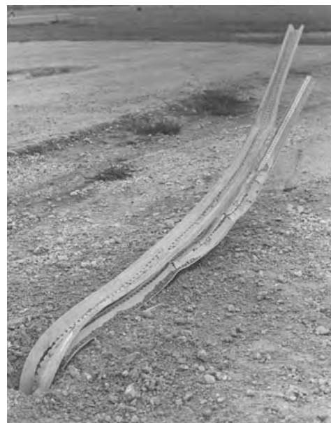
Figure 3-10: U-channel system that did not perform as intended
