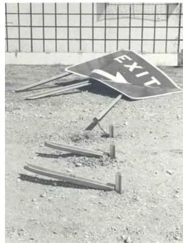
Figure 2-6: U-channel system that performed as intended
