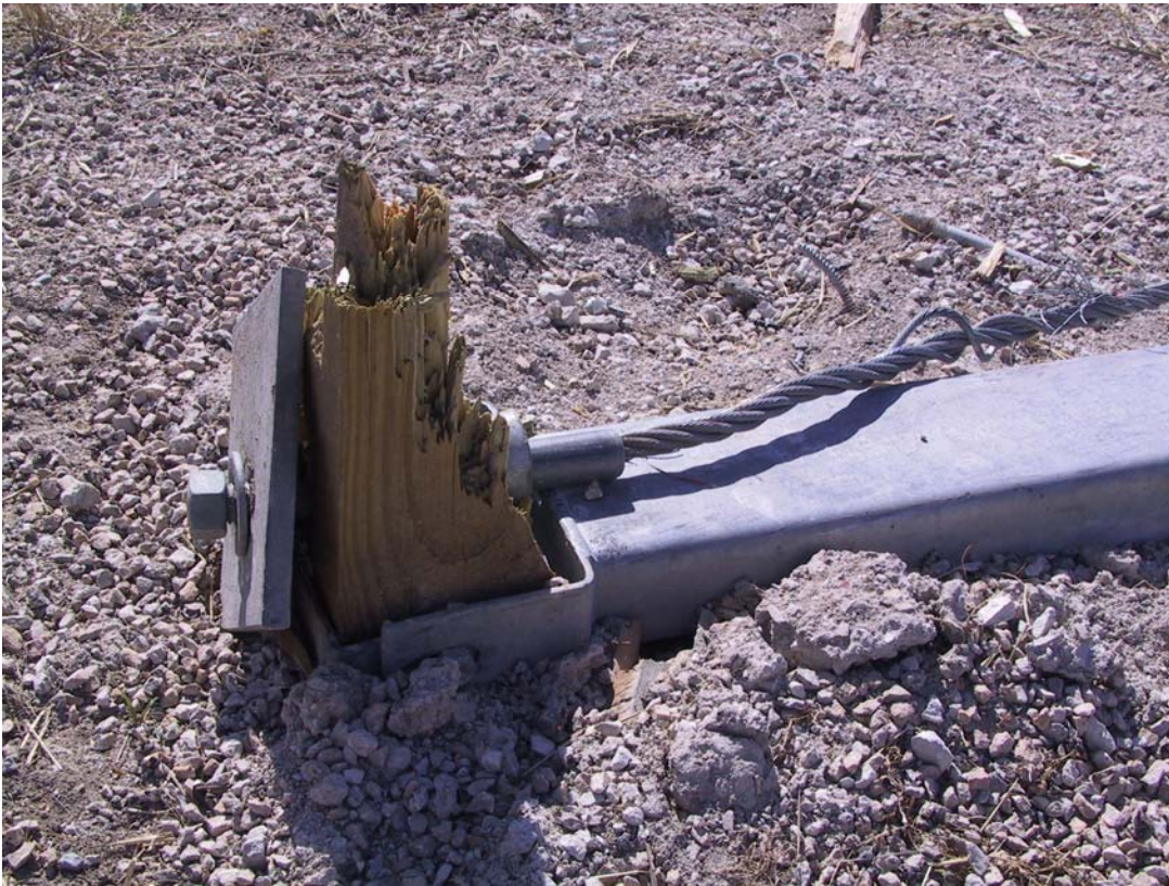
Figure D6: An Example of an ET-2000 Impact Observed During the Pilot Test.
