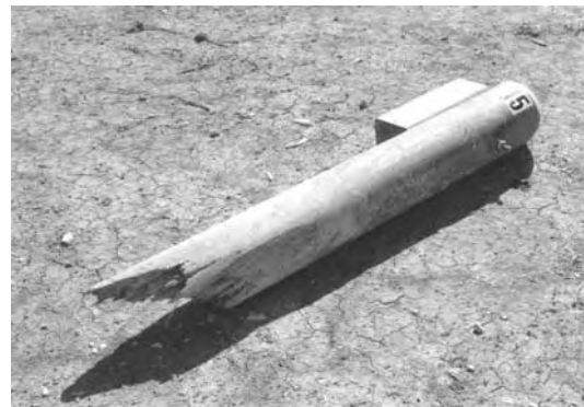
Figure 1-6: Fractured wooden post
