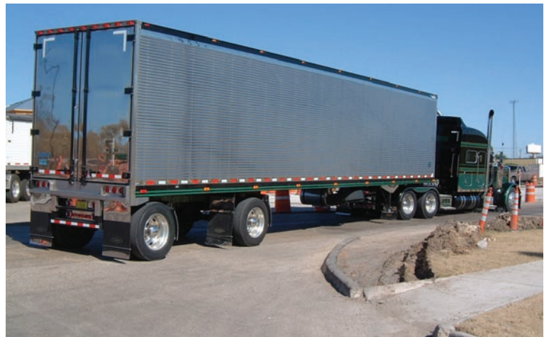
Figure 1. Inadequate Intersection Design for Trucks.
