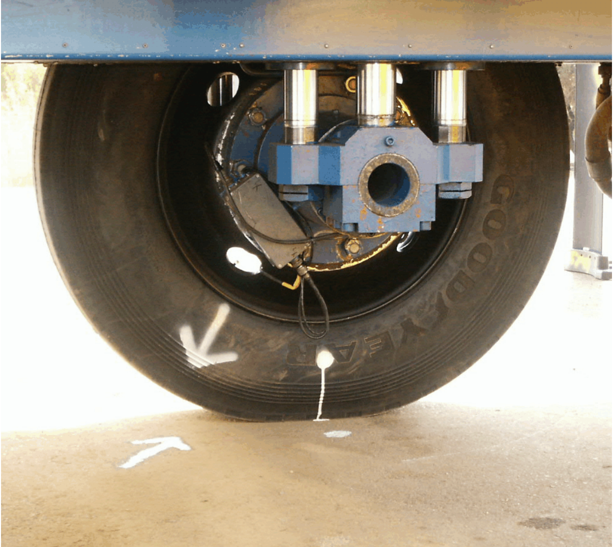
Figure 3.7. Marks Used to Position Tire for a Test Run.
