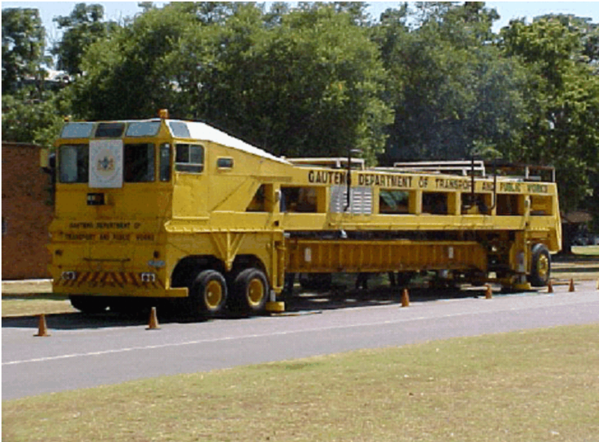
Figure 2.1. Heavy Vehicle Simulator Used for Tire Testing (de Beer and Fisher, 2002).
