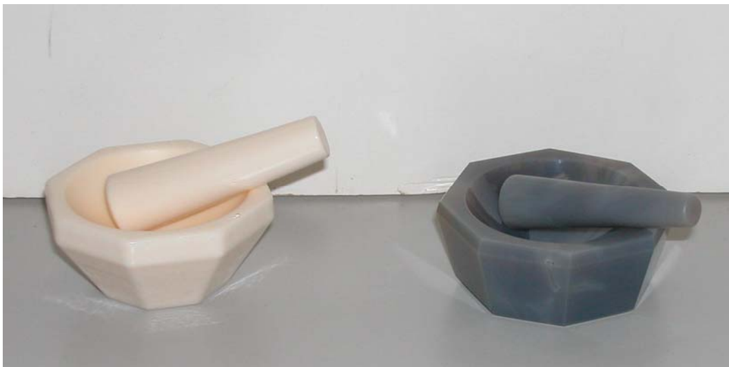
Figure A16. Aluminum Oxide (left) and Agate Mortars and Pestles for Sand Reduction.
