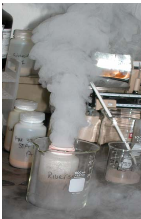
Figure A4. Removal of Organic Matter Often Results in a Violent Reaction.
