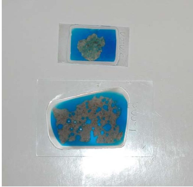
Figure A1. Typical 1 X 2 Inch and 2 X 3 Inch Thin Sections.
