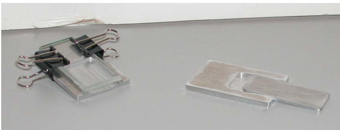
Figure A17. Aluminum Holders Used for Side Loading Sand and Silt into X-Ray Unit.
