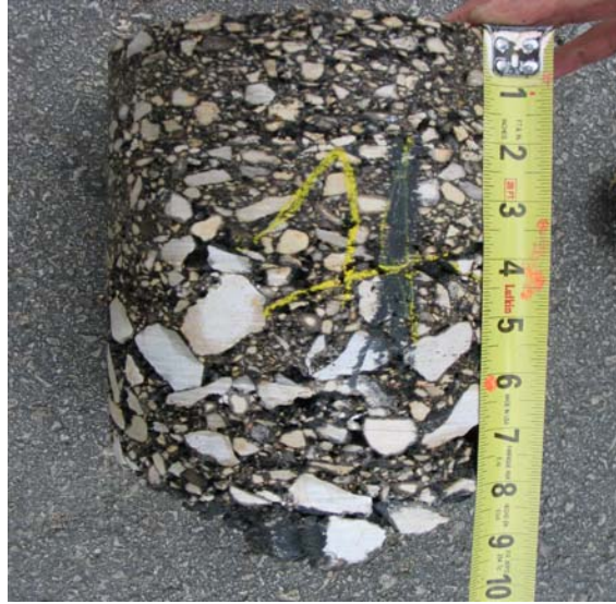
Figure 27. Poorly Compacted Core from the IH 35 Detour Failure.
