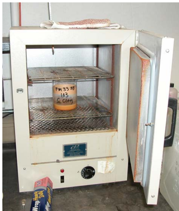
Figure A8. Oven Set at 60 °C for Drying Sand, Silt, and Coarse Clay Fractions.
