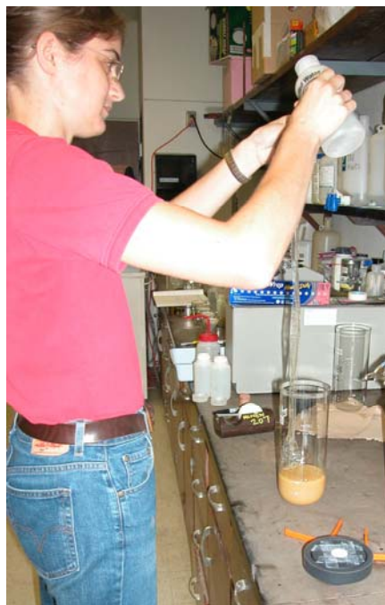
Figure A12. Clay-Water Suspension Being Placed in Freeze Dryer Flask.
