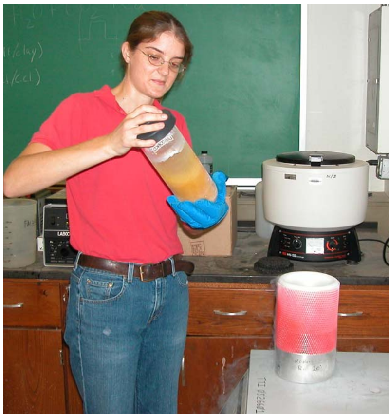
Figure A14. Rotation of Freezing Suspension to Achieve Inverted Cone Shape.
