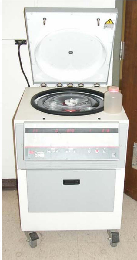
Figure A7. IEC Centra GP8R Centrifuge Used to Separate Silt and Clay Fractions.
