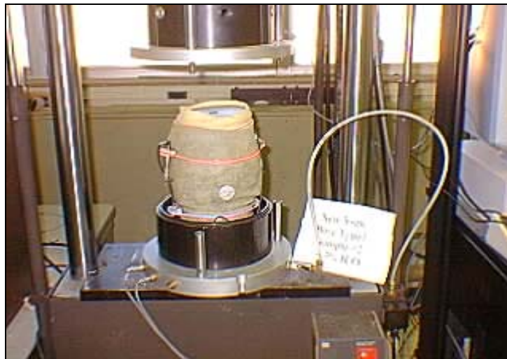
Figure 54. Failed New York Base in Resilient Modulus Test (Kancherla, unpublished data).
