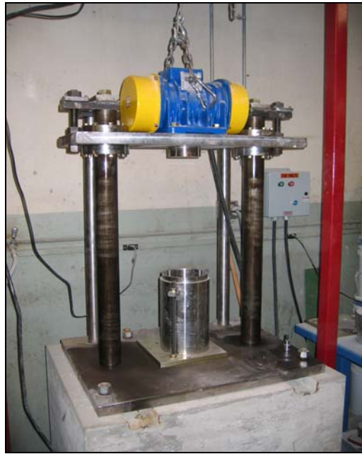
Figure 55. TTI's Prototype Vibratory Laboratory Compactor.
