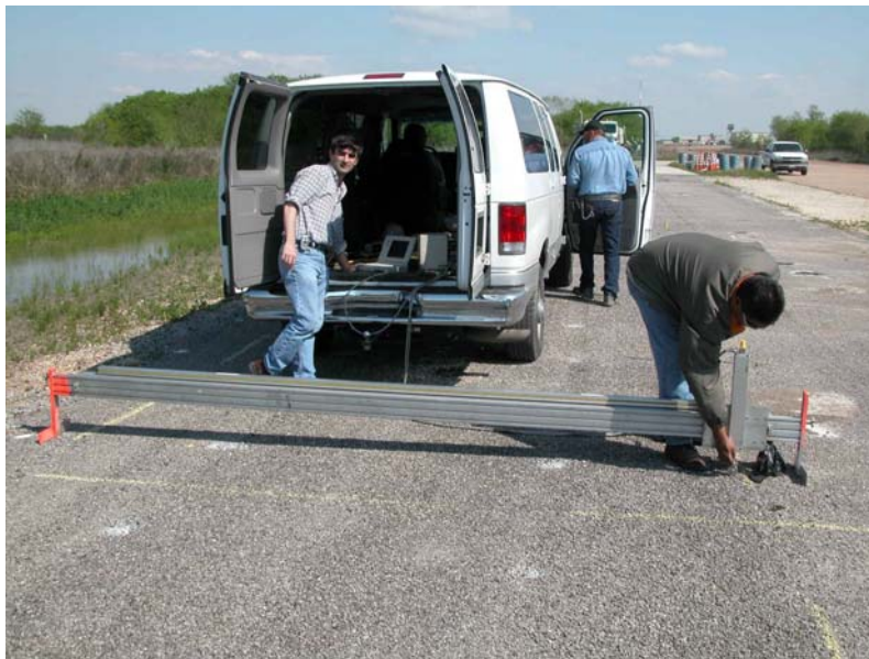
Figure 49. Rut Determination on Test Sections.
