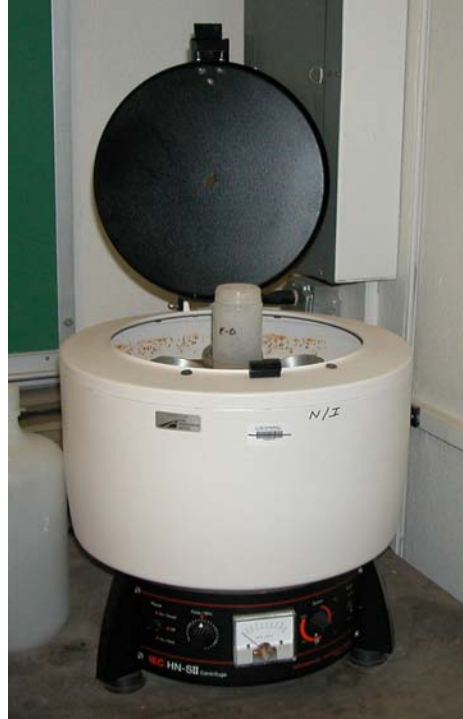
Figure A5. Centrifuge Used to Aggregate the Sample Prior to Decanting Supernatant.
