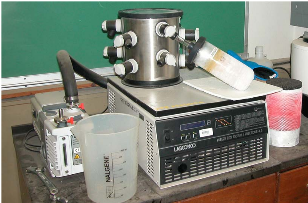
Figure A15. White Coating of Ice on the Flask, Indicative of a Successful Freezing Job.
