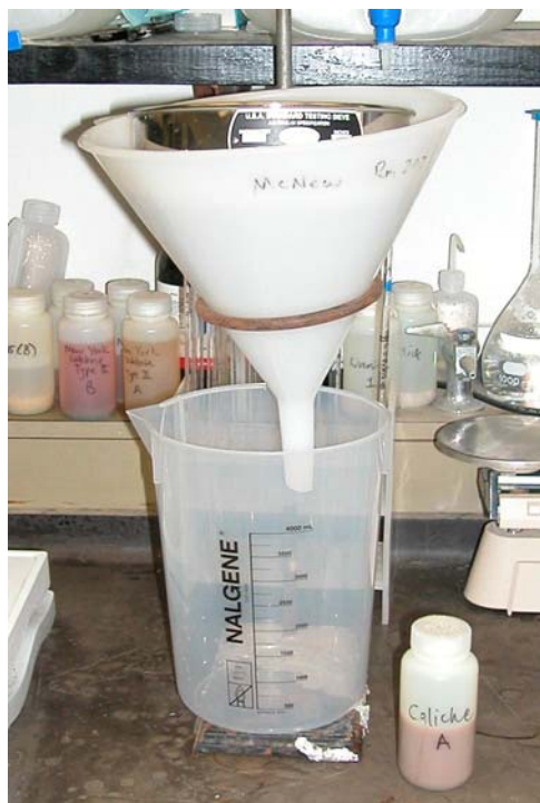
Figure A6. Ring Stand, Funnel, and Sieve Assembly Used for Sand Fractionation.
