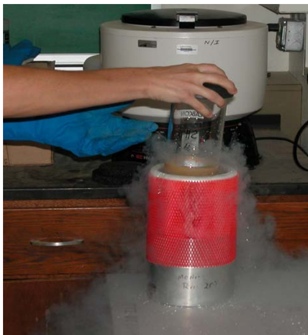
Figure A13. Freezing Clay-Water Suspension Using Liquid Nitrogen.
