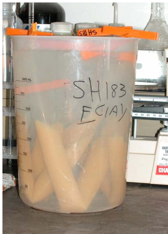
Figure A10. Fine Clay Placed in Dialysis Tubing to Remove Salt by Osmosis.
