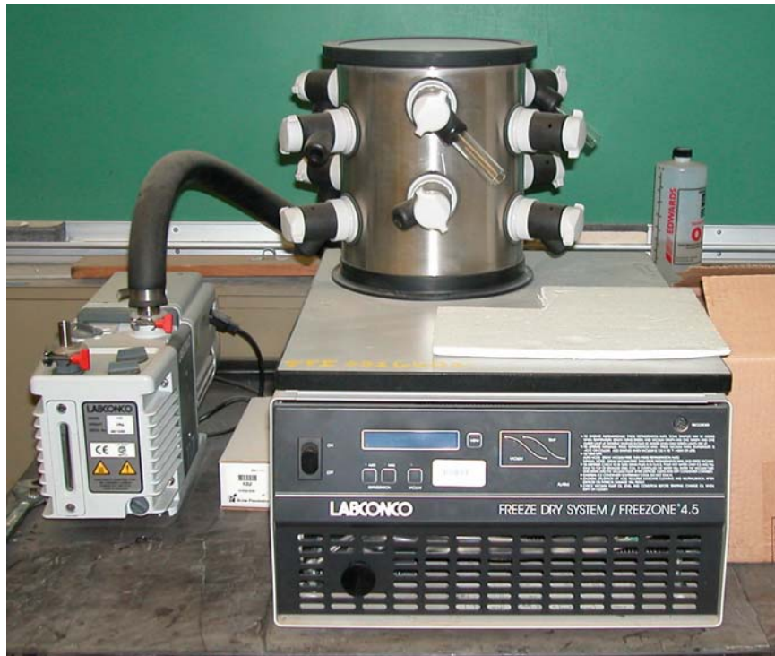
Figure A11. Freeze Dryer Used to Remove Water from the Fine Clay Fraction of Samples.
