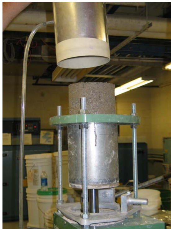
Figure 53. Extruding Item 245 Bases Directly into Membranes.
