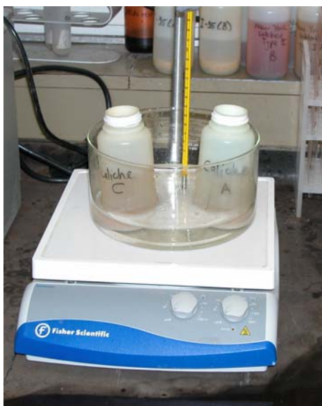
Figure A3. Caliche Sample in Water Bath for Carbonate Removal.
