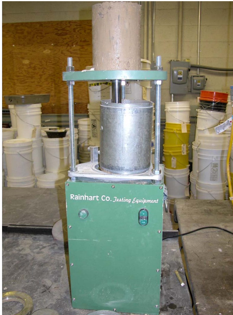
Figure 6. Extrusion of Specimen from the Compaction Mold.
