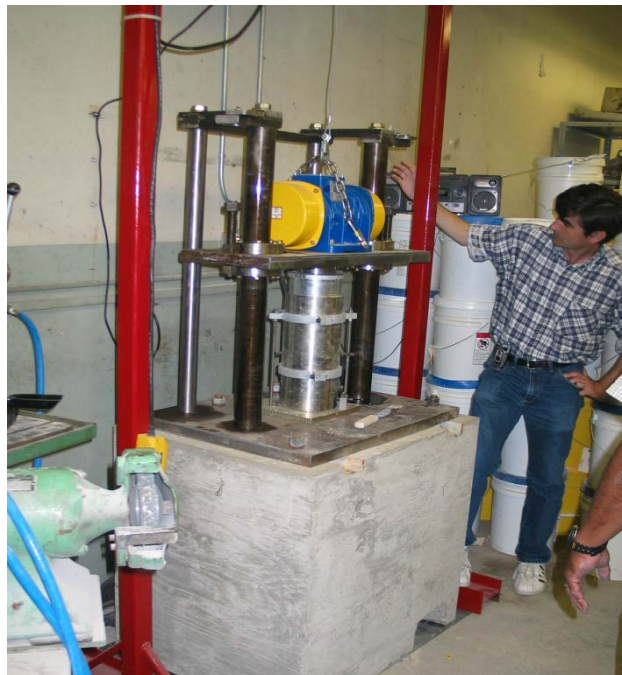
Figure 25. TTI's New Base Vibratory Compactor.
