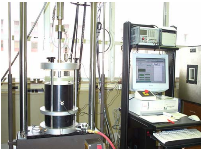
Figure A-1. Test setup of Resilient Modulus. Figure A-2. Specimen prepared for Testing.
