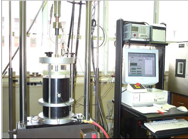
Figure 3. Test Setup for Resilient Modulus.
