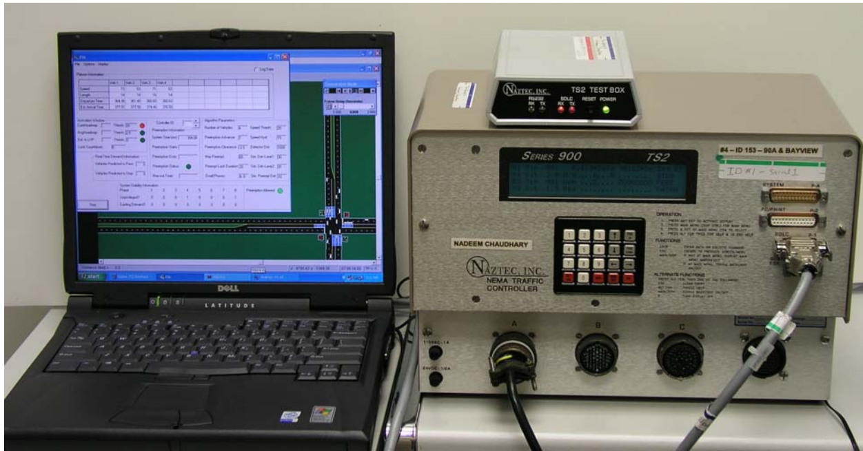
Figure 7. Software Using Controller-in-loop Simulation.
