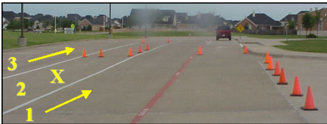
Figure 34. Placement of Traffic Cones to Create a Dual-Lane Queue.
