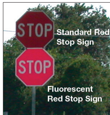
Figure 2. Fluorescent vs. Standard Red Stop Sign.
