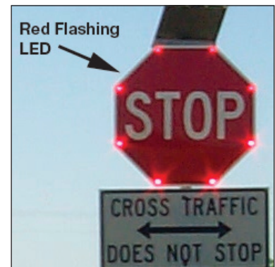
Figure 3. Red Flashing LED Stop Sign.
