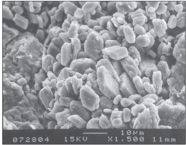
Figure 3. Scanning Electron Microscope Image of Very Small Gypsum Crystals.
