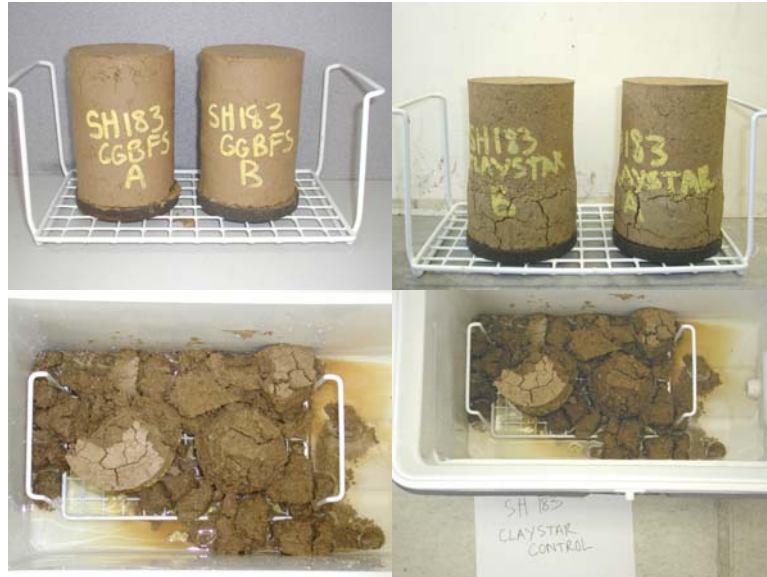
Figure 37. Clockwise from Top Left: 5% GGBFS & 1% Lime, ClayStar, Control Cured as GGBFS: Lime, Control Cured as ClayStar (treated at completion of 10-day capillary rise and untreated fell apart after Day 1).
