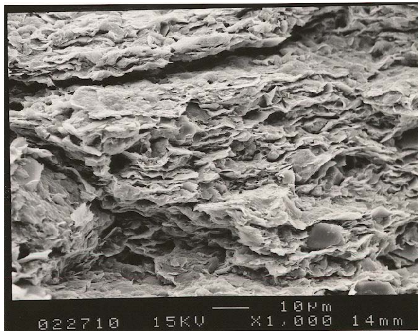
Figure 10B. SEM Image of Natural Clay Rich Soil. (The crinkly masses are smectite grains. Note the absence of long needle-shaped crystals.)
