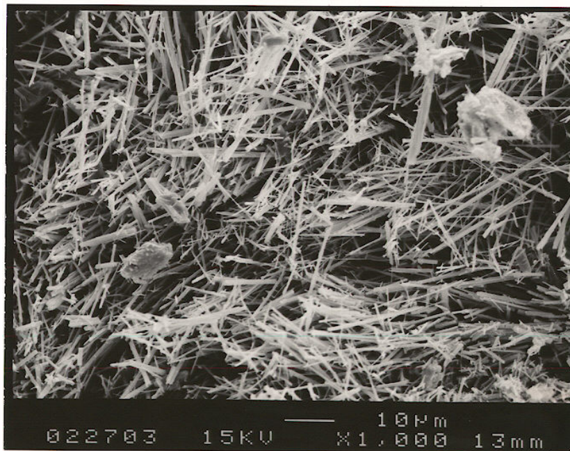
Figure 13B. SEM Image from Sample E-1 LTSa Shows Acicular Prismatic Crystals Which Are Typical of Ettringite. (This is an expansive reaction product of lime and gypsum.)
