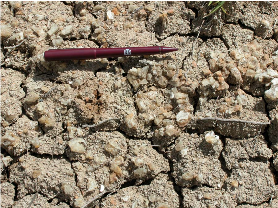
Figure 3. White Crystals below the Mechanical Pencil are Gypsum Crystals in Drainage Ditches on FM 201.
