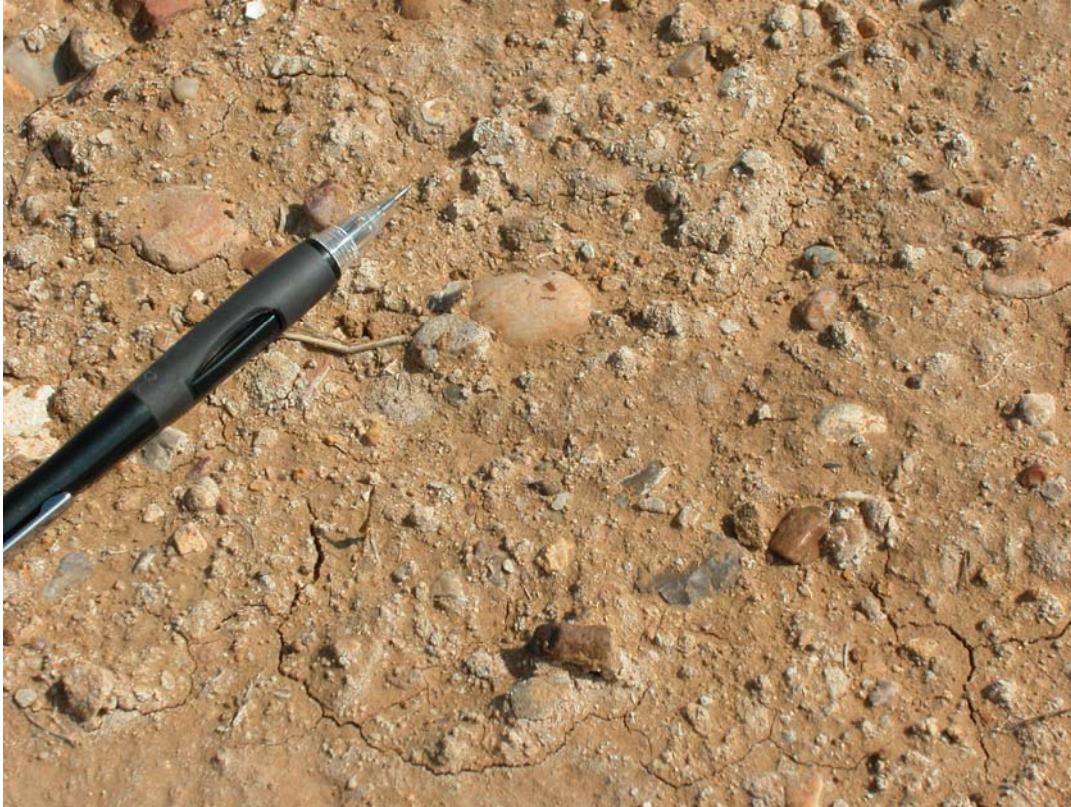
Figure 23. Mechanical Pencil Points to Small Gypsum Crystal. (Note also the white patches.)
