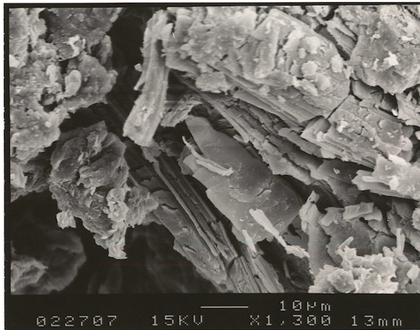
Figure 11B. SEM Image from Sample E-1B Showing Gypsum Crystals in the Untreated Subgrade.
