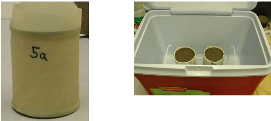
Figure 6. Sample Preparation for 3-D Swell Measurement.
