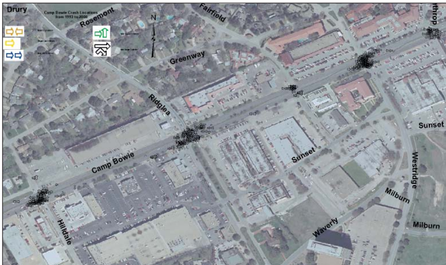
Figure 1. Crash Density on Corridor with Low Access Density.
