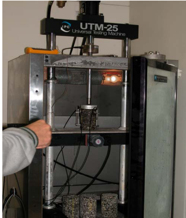
Figure 2.3. UTM Machine Used for Simple Performance Tests.
