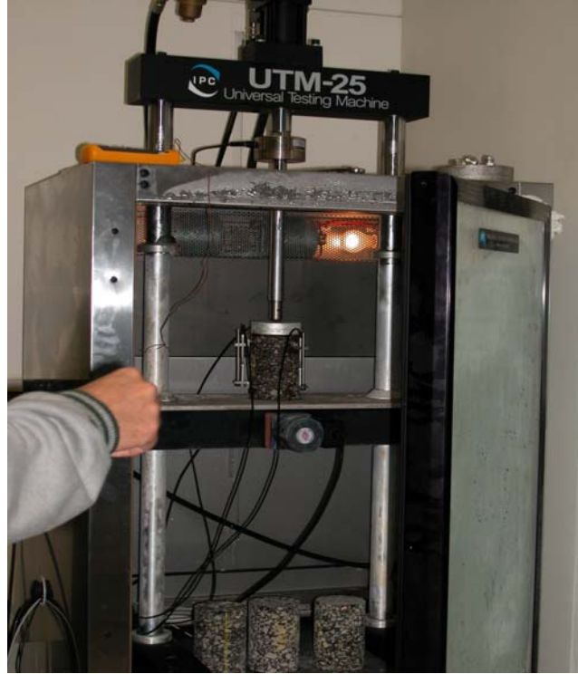
Figure 4.1. Dynamic Modulus Testing Setup.
