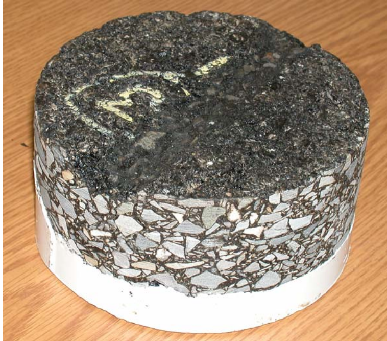
Figure 8. Modified Roadway Core Specimen after APA Testing.
