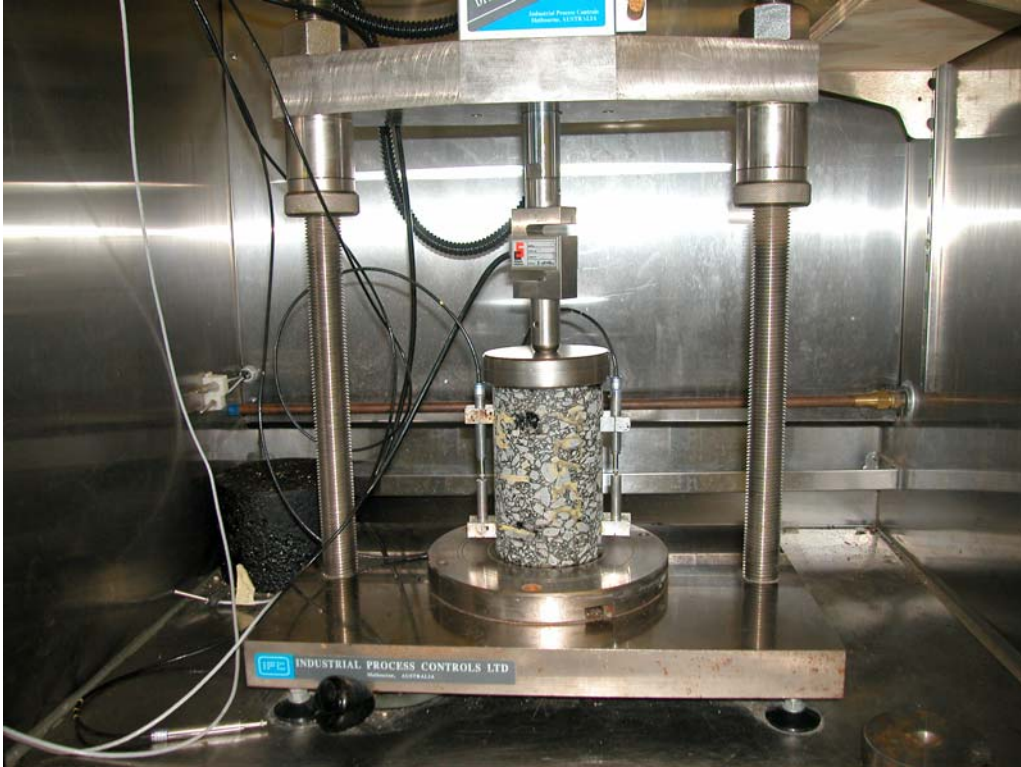
Figure 10. Dynamic Modulus Testing Setup.
