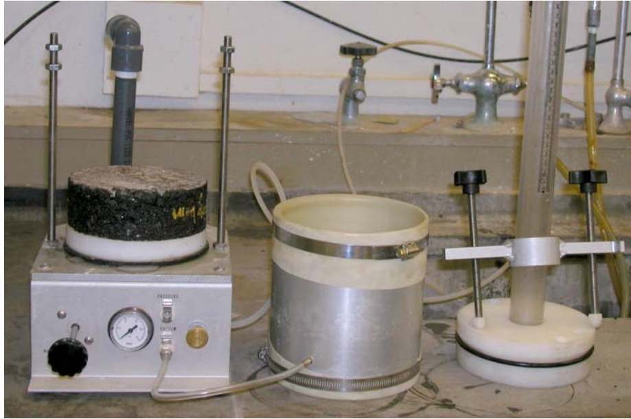
Figure 4. Florida Permeability Test Apparatus.
