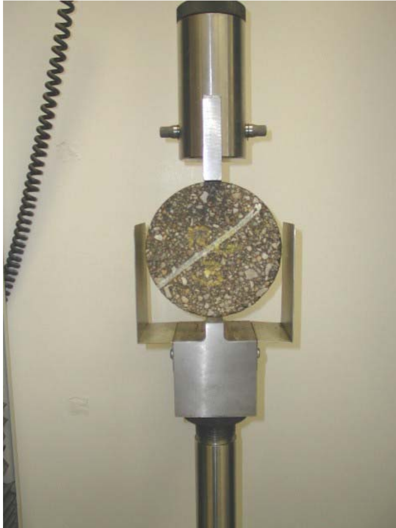
Figure 9. Indirect Tensile Strength Test Setup.
