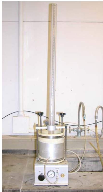
Figure 5. Florida Permeability Test Setup.
