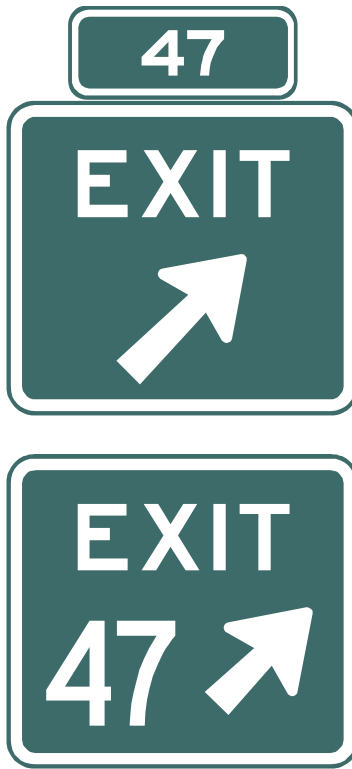
Figure 2. Exit Numbering for Exit Gore Signs.
