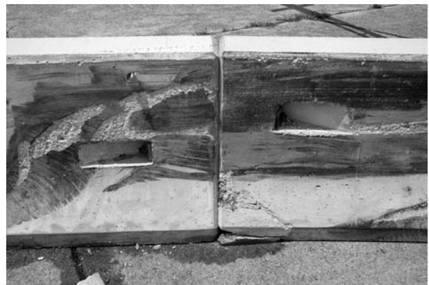
Figure 15. Installation after Test 441623-1.
