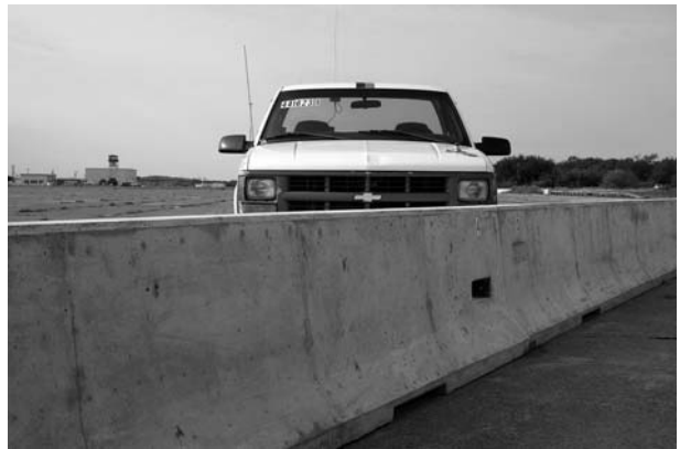
Figure 12. Vehicle/Installation Geometrics for Test 441623-1.
