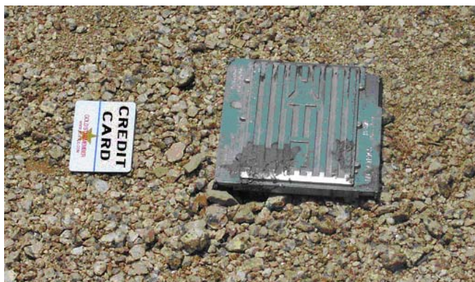
Figure 20. HI-STAR Data Collector (Credit Card as Size Reference).
