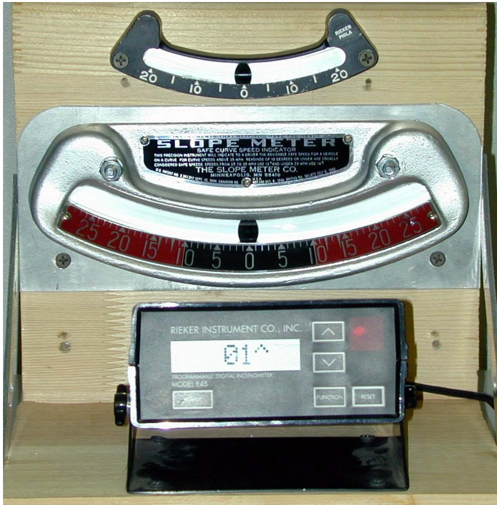
Figure 10. Ball Bank Indicators.
