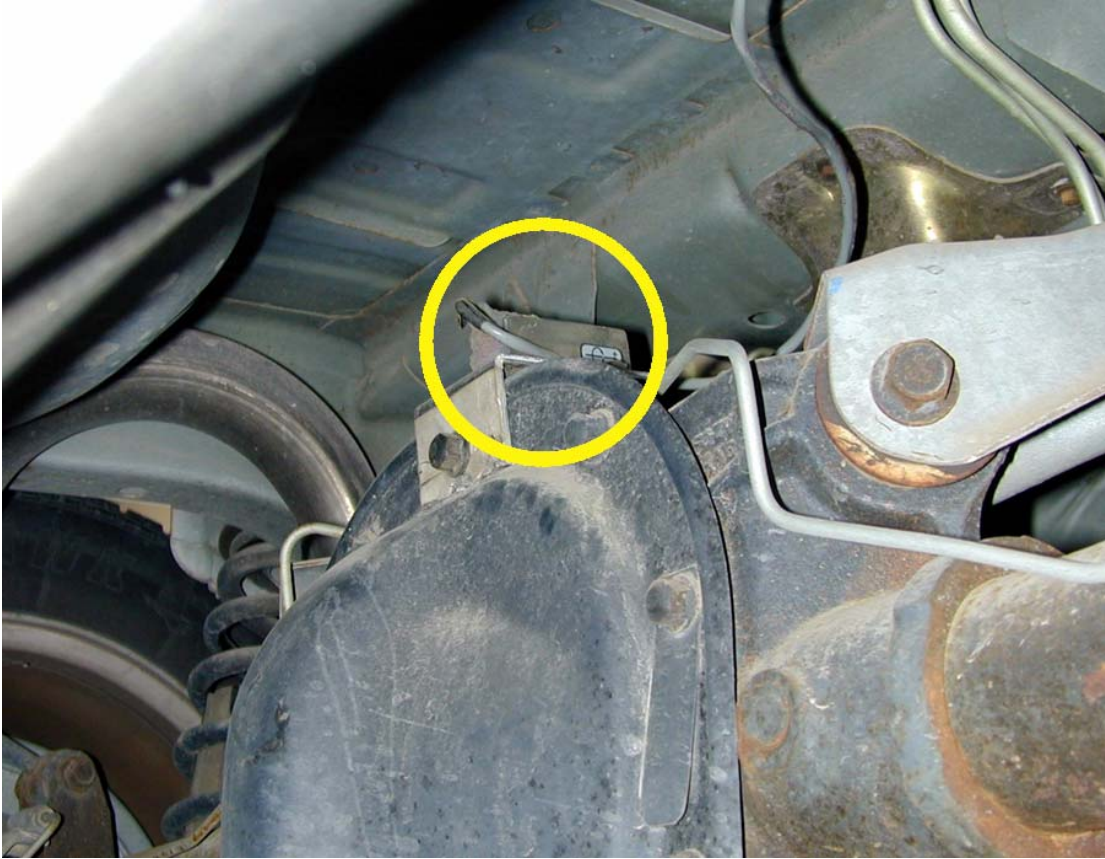
Figure 13. Roll-Rate Sensor Position on the Fixed Suspension.
