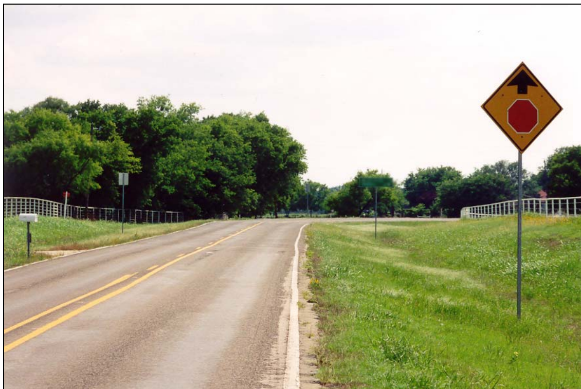
Figure 5-2. STOP AHEAD Sign on Intersection Approach in Advance of Curve.
