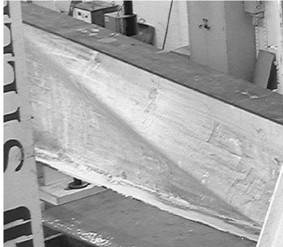
Figure 71. Photograph of Tension Field in the 90-Degree Rounded Specimen.
