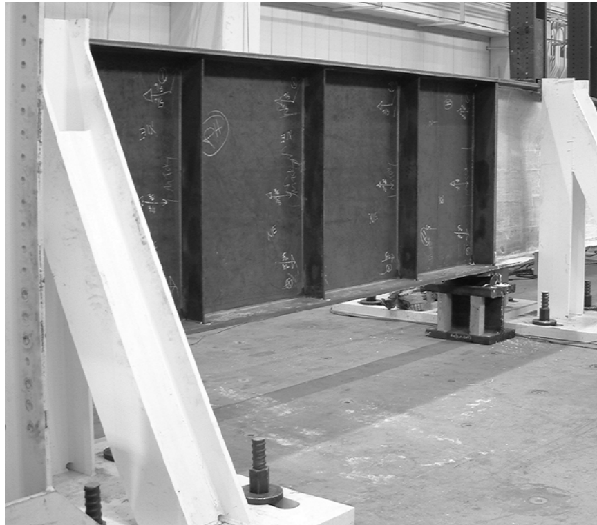
Figure 61. Photograph of Heavily Stiffened Backspan and Interior Rocker Support.
