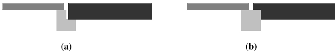
Figure 1. (a) Stepped Bent Cap. (b) Dapped Girder.
