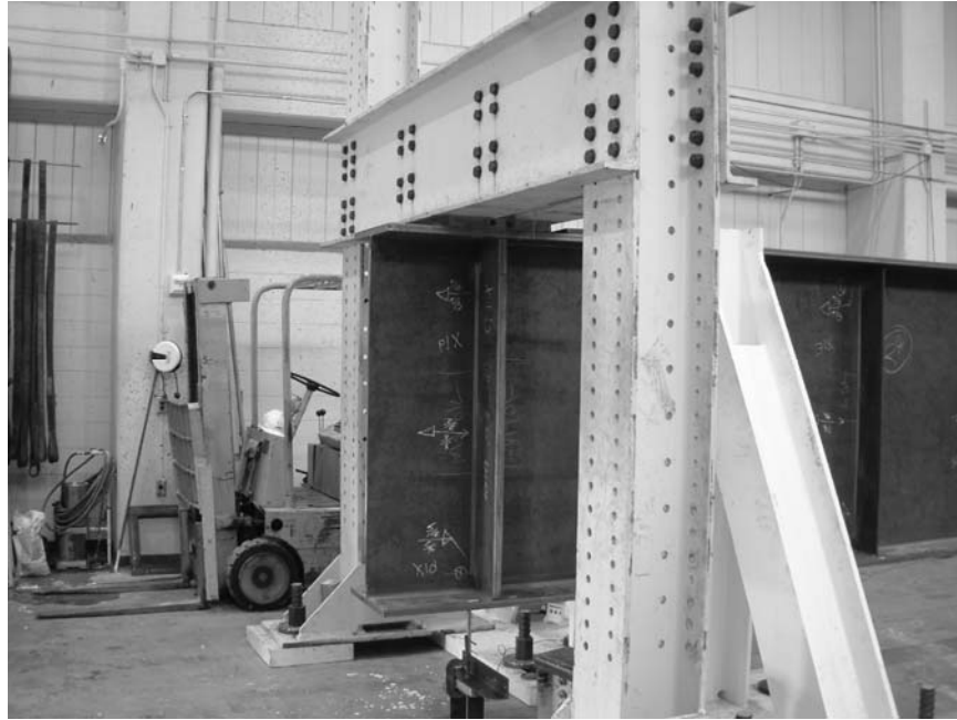
Figure 62. Photograph of Backspan End-Support Configuration.
