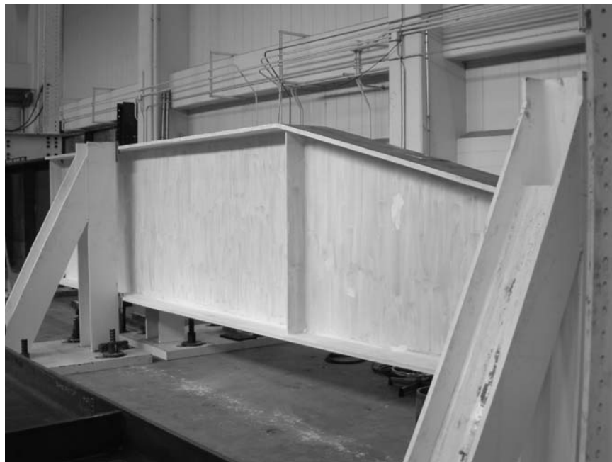
Figure 65. Pretest Photograph of Stiffened Tapered Specimen.
