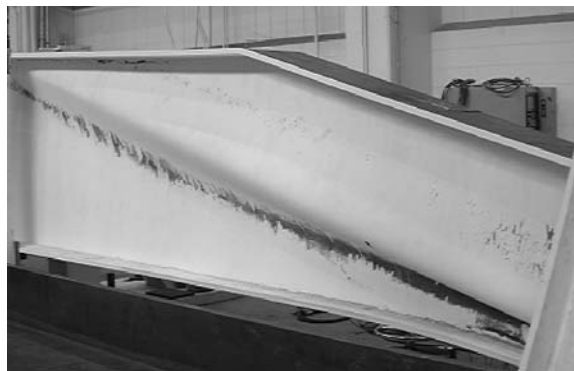
Figure 73. Photograph of Tension Field in the Unstiffened Tapered Specimen.
