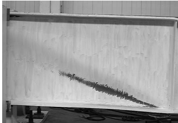
Figure 75. Photograph of Tension Field in the Stiffened Tapered Specimen.
