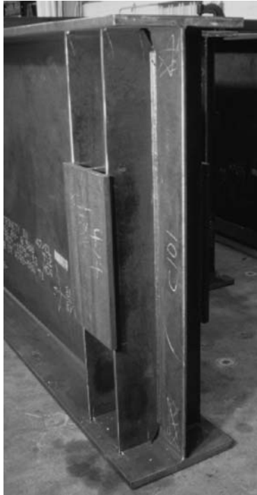
Figure 33. Photograph of WT Shape Welded to Stiffeners at End of Specimens.
