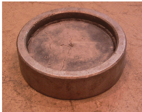
Figure 3.6. Neoprene Pad and Steel Retaining Ring.
