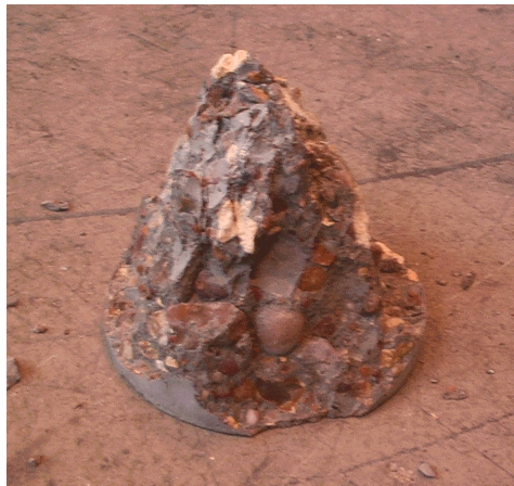
Figure 3.8. Compression Cone Failure.
