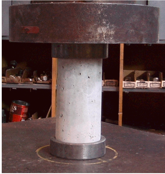
Figure 3.7. Compressive Strength Test.
