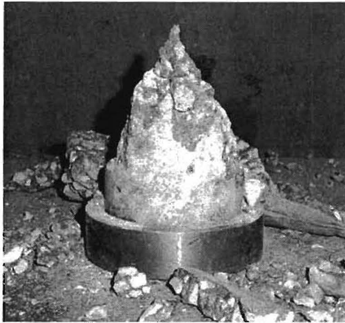
Figure 4.2. Failure of Compressive Strength Specimen.
