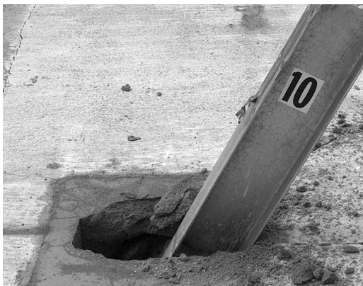
(c) Steel Post in Grout-Filled Leave-Out
