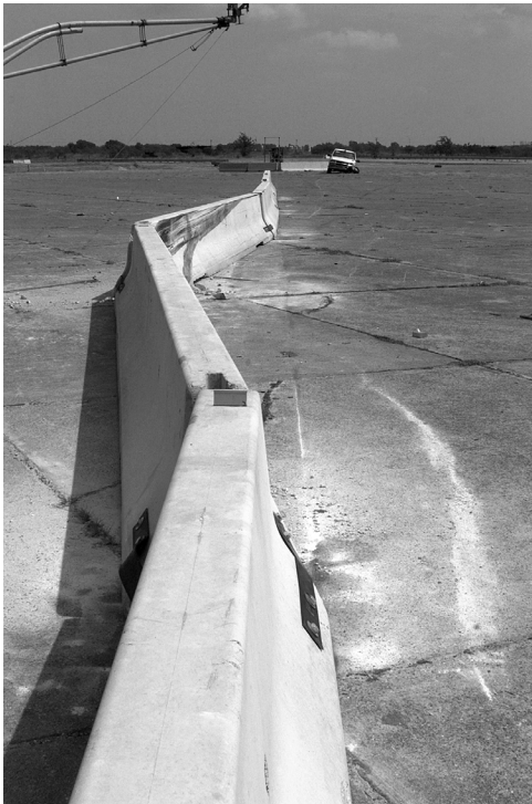
Figure 16. Grid-Slot Barrier with Steel Strap Retrofit After Crash Test.
