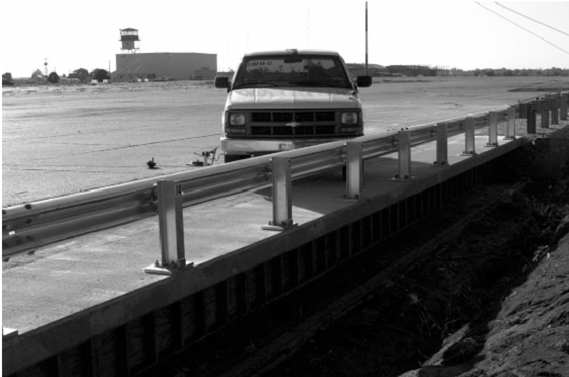
Figure 1. T6 Bridge Rail Prior to Crash Test.
