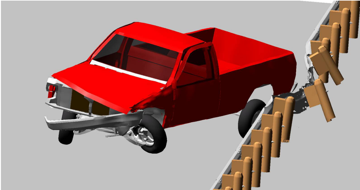
Figure 30. Vehicle Pocketing During Impact of Wood Post System in Rigid Mow Strip.
