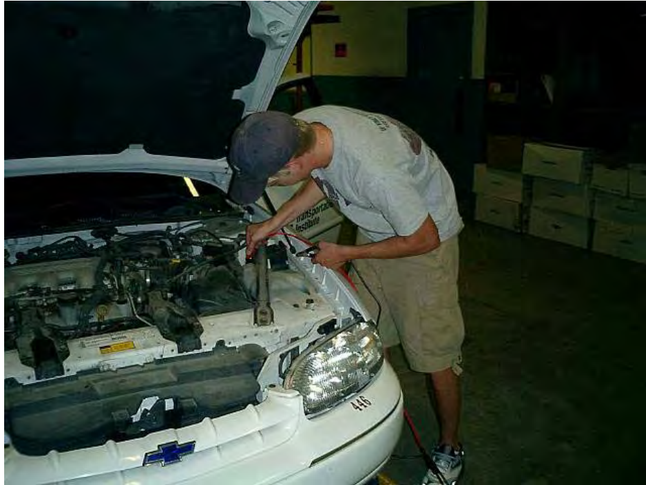
Figure 12. Attachment of Voltage Regulator to Battery.
