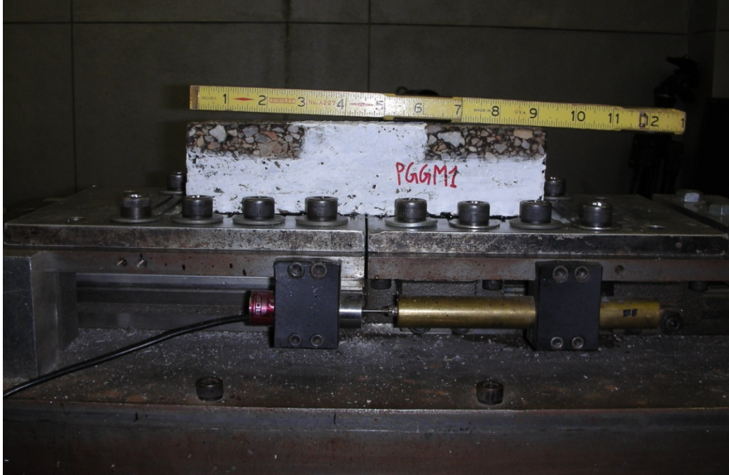
Figure 4-8. Test Setup of Medium-Sized Specimen with Small Overlay Tester.
