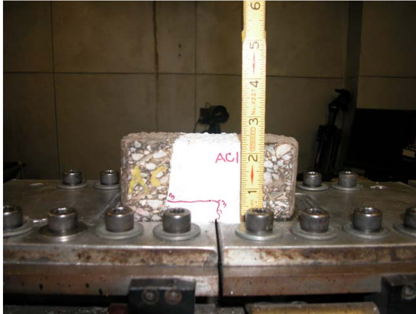
Figure 4-7. Testing of Small Specimen with Small Overlay Tester.
