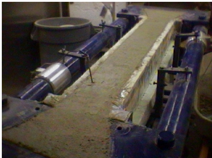
Figure D-1 Cracking Frame.
