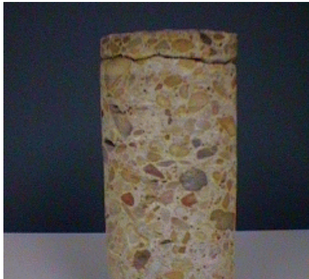
Figure 6. Delamination of Unspalled Core (13).
