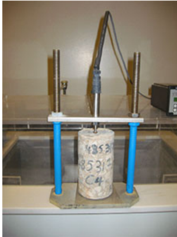
Figure 9. AASHTO TP-60-00 COTE Test Frame with LVDT.
